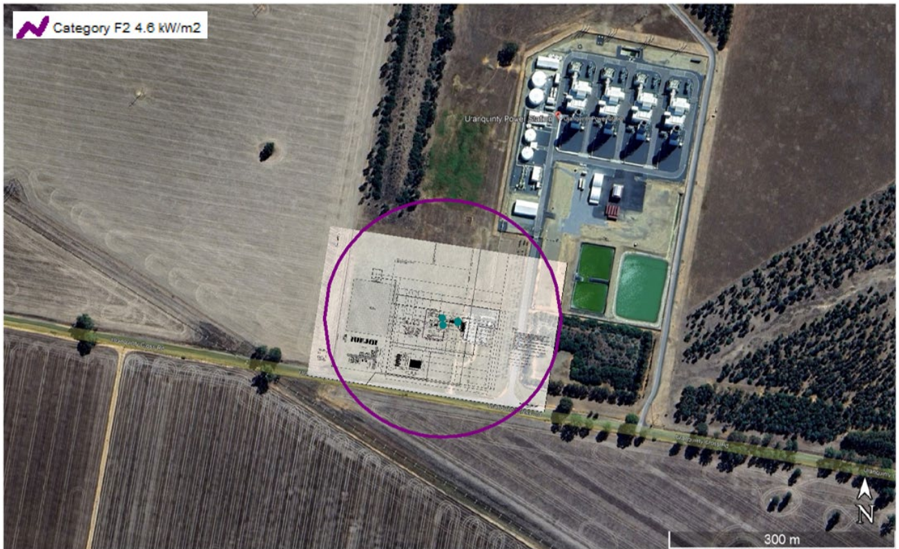
Figure 6.10 Fireball scenario, full bore rupture – 4.7 kW/m 2 effect zone, 1.6/F weather condition
