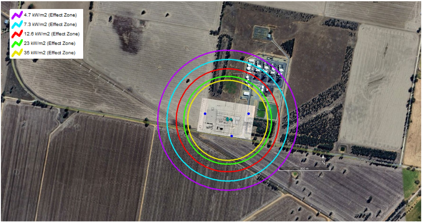
Figure 6.2 Scenario 2: Compressor and inlet piping, full bore rupture – Jet fire effect zone, 1.6F weather condition
