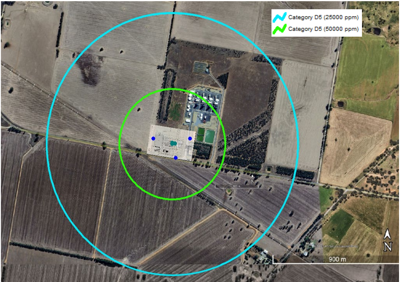
Figure 6.6 Scenario 2: Compressor and inlet piping, full bore rupture – Flash fire effect zone, 5.1D weather condition
