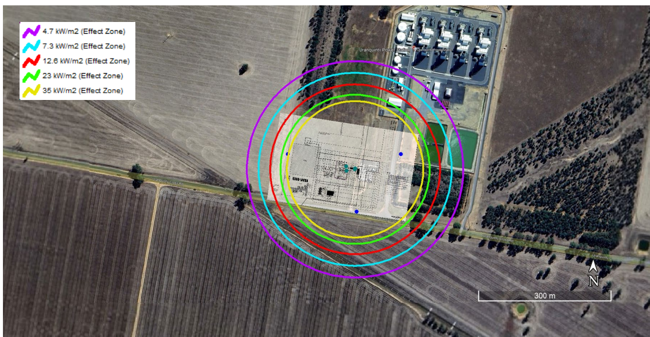
Figure 6.4 Scenario 4: Compressor discharge piping to pipeline take off, full bore rupture – Jet fire effect zone, 5.1D weather condition
