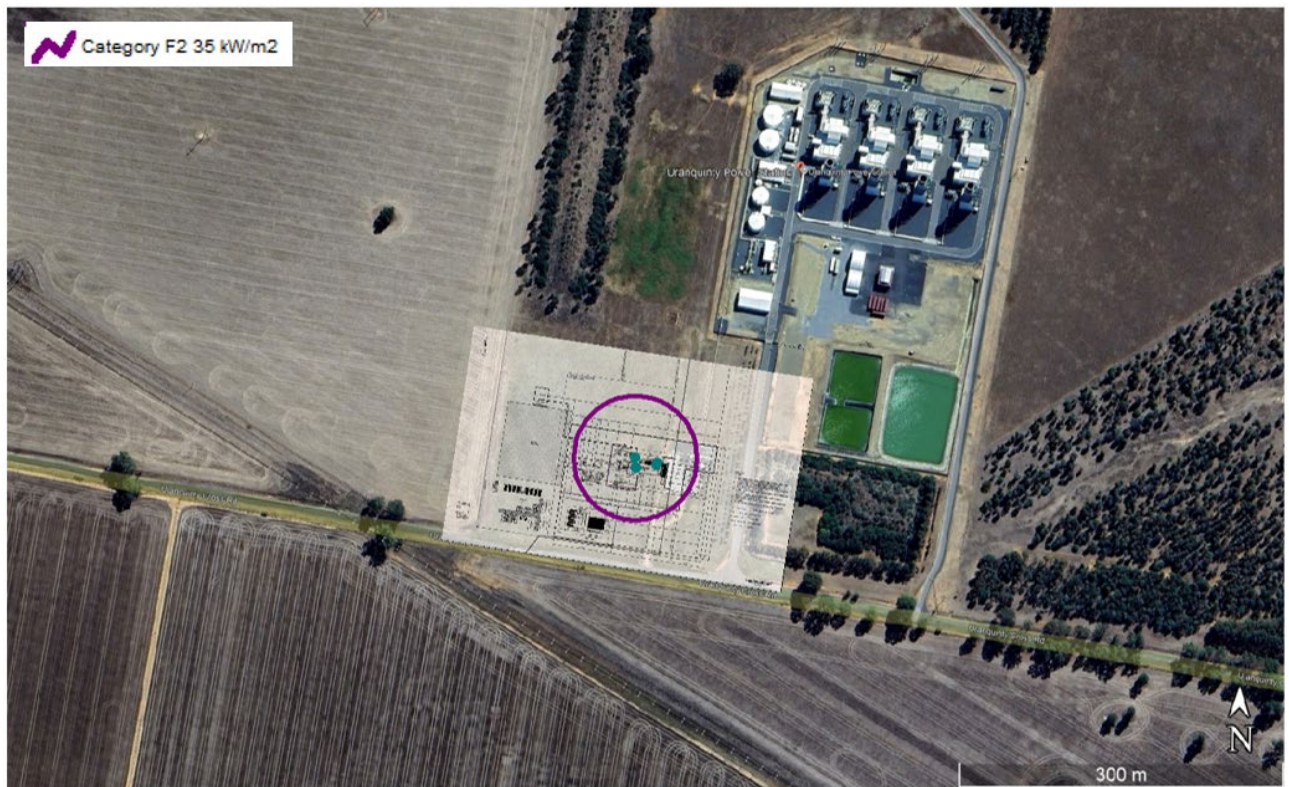
Figure 6.11 Fireball scenario, full bore rupture – 35 kW/m 2 effect zone, 1.6/F weather condition
