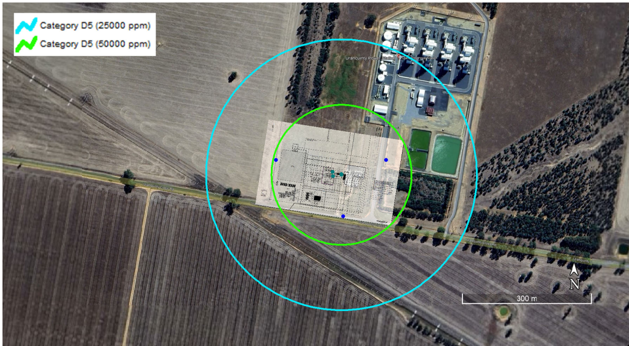
Figure 6.8 Scenario 4: Compressor discharge piping to pipeline take off, full bore rupture – Flash fire effect zone, 5.1D weather condition
