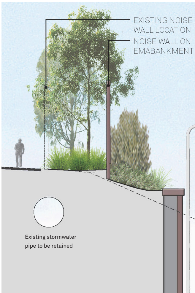
Figure 65 Proposed noise wall design including retaining of earth to minimise slope for planted areas, and planter bed to be of adequate width to accommodate substantial landscape treatment
