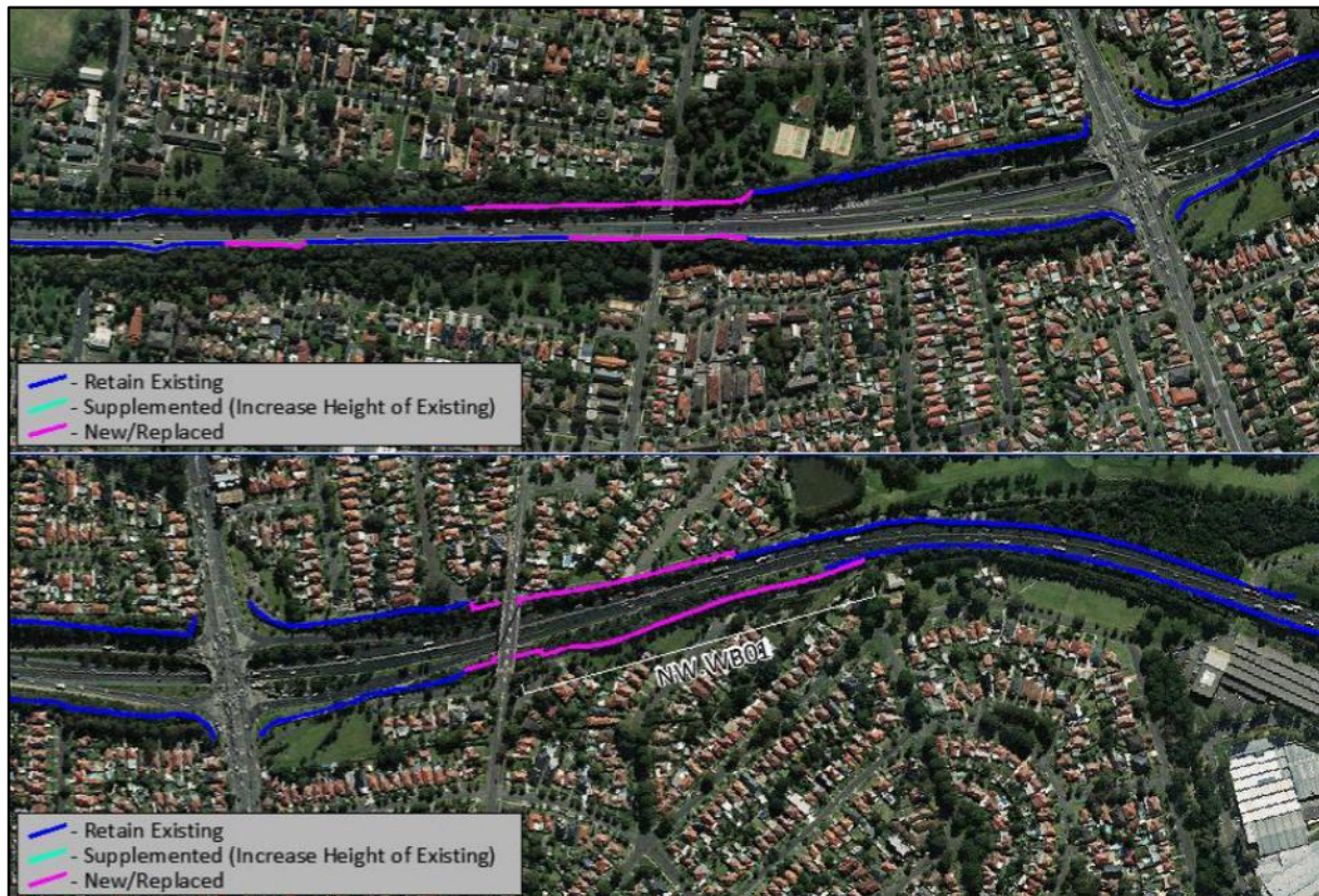
Figure 7 Recommended noise barriers
