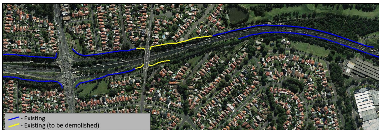
Figure 5 Existing noise barriers to be replaced (near Cooloongatta Road Bridge)
