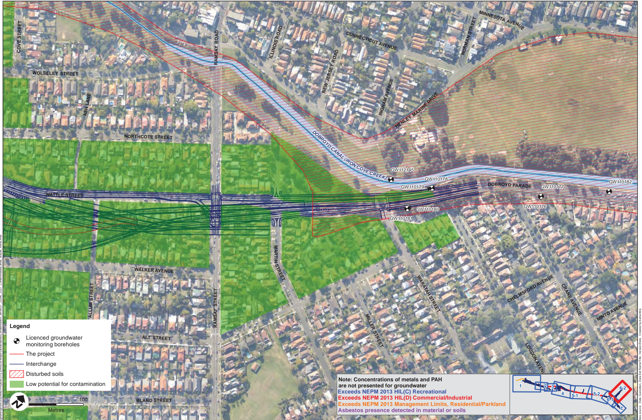
Figure 4-8.2 Investigation locations, exceedances, summary of contaminated land survey and land uses Section 6-2 Wattle street
