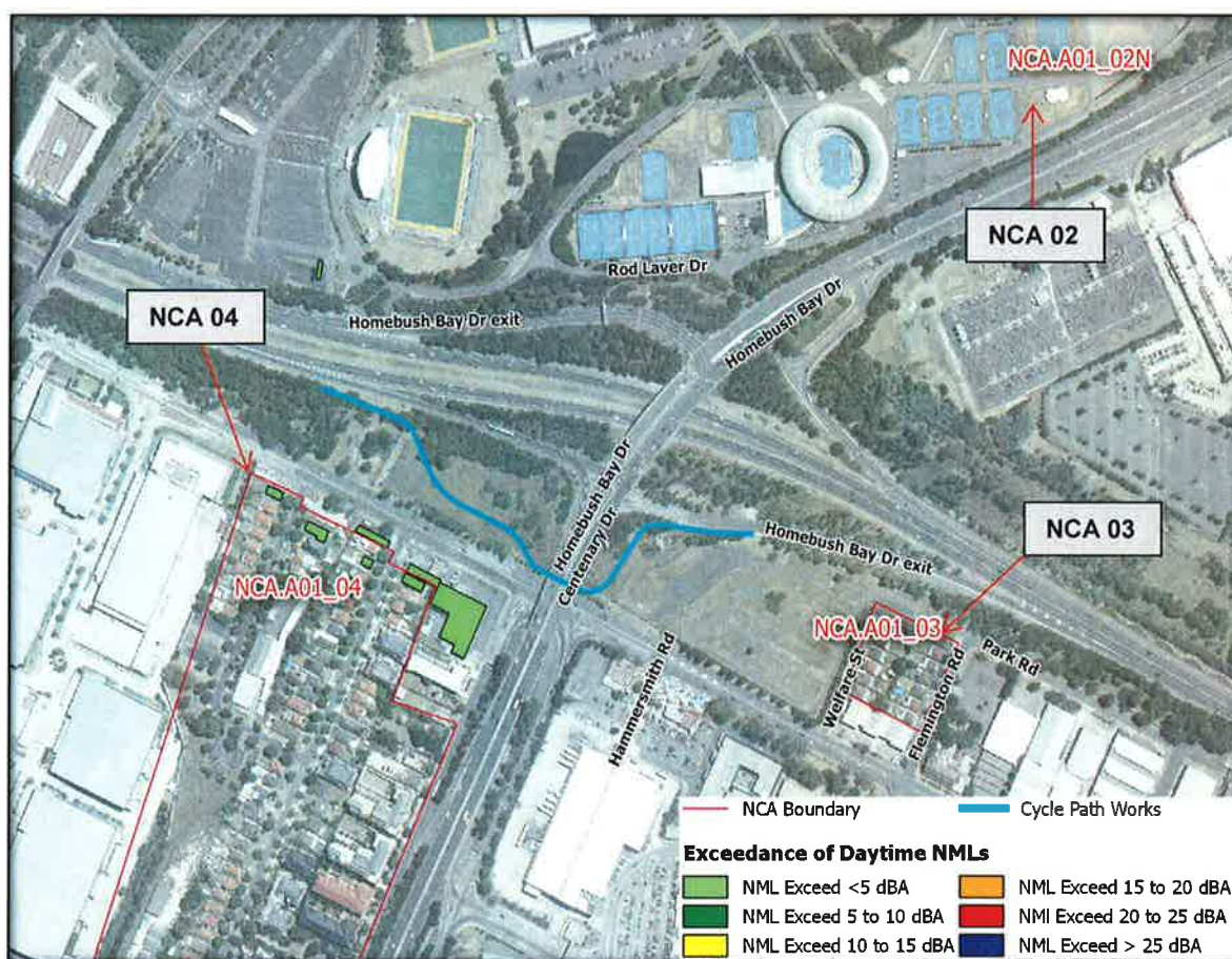
Figure 3: Noise Catchment Areas Adjoining the Homebush Bay Drive Interchange (Source: CNIA)
