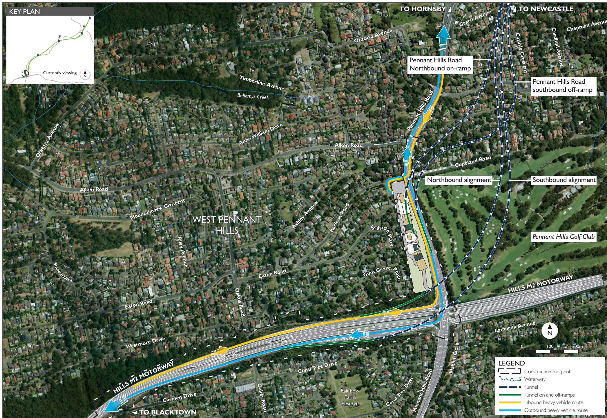
Figure 9-16 Southern interchange compound access arrangement C5-5
