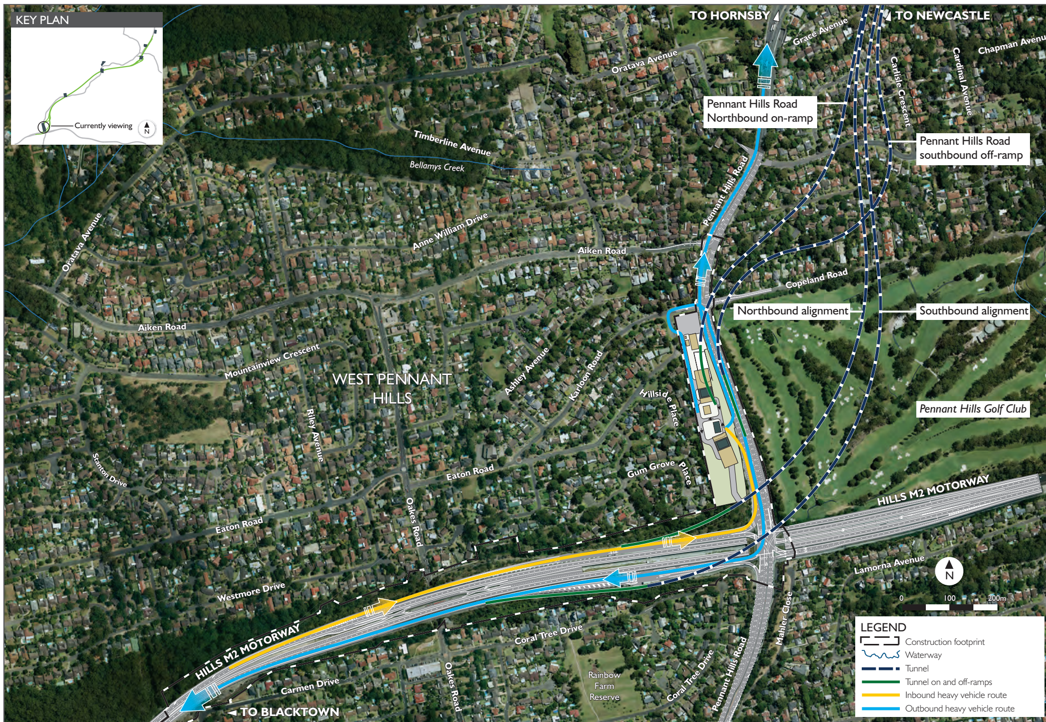
Figure 9-15 Southern interchange compound access arrangement C5-4
