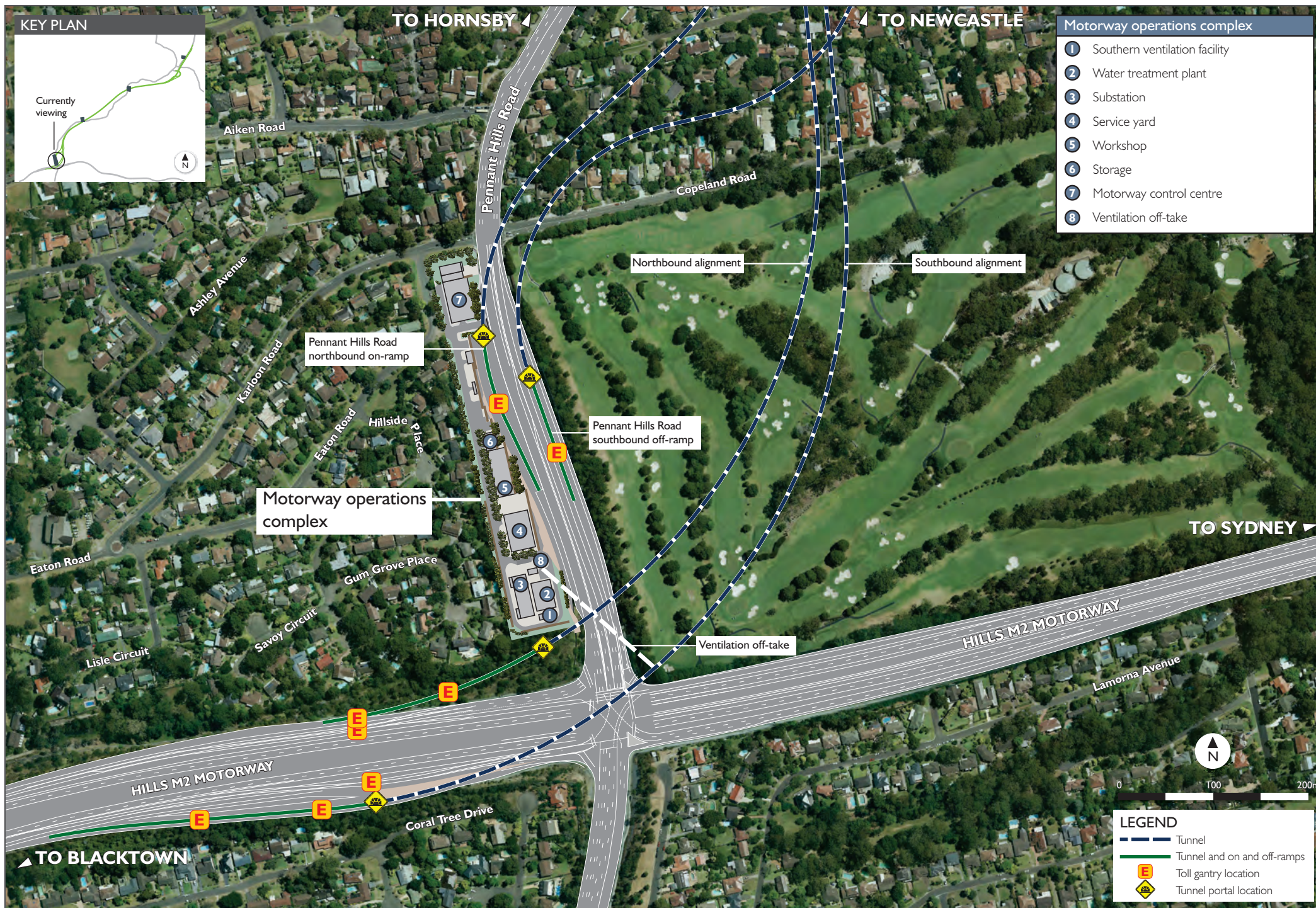
Figure 4-1 Southern ventilation off-take location
