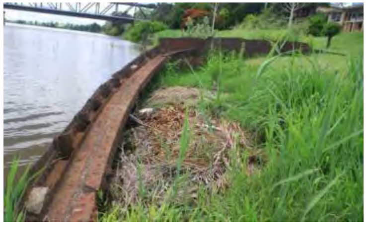
Photograph 24: View east along port quarter to bulk head behind bow with intact topside of hull and reed growth inside hull
