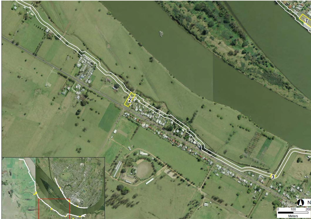
Figure 6c: Levee construction work zones and stockpile areas
