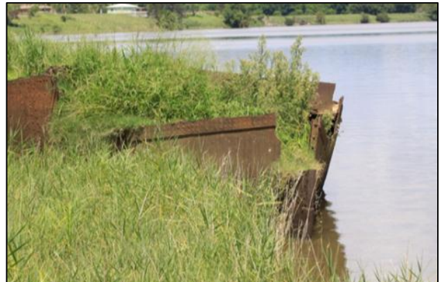
Plate 58: East facing photograph of the stern of SS Induna (FMW29) (left) and (right) bow area where bow was removed for nearby memorial (Source: Comber Consultants).
