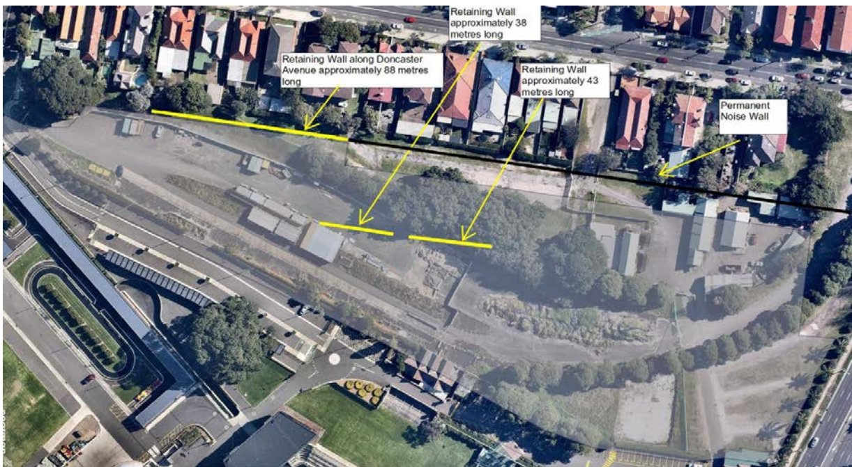
Figure 6 Retaining wall construction
