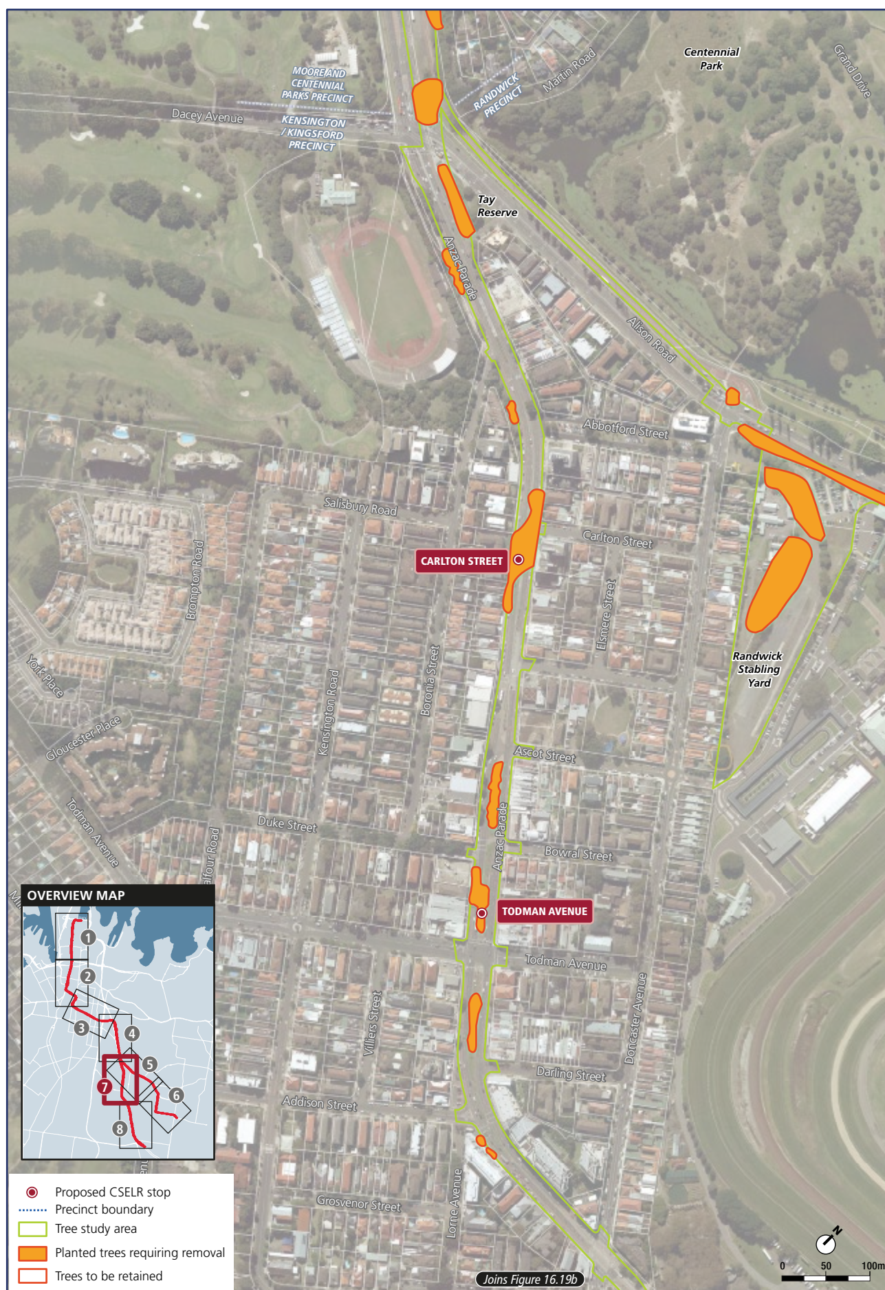
Figure 16.19a Impacts to planted trees – Kensington/Kingsford Precinct
