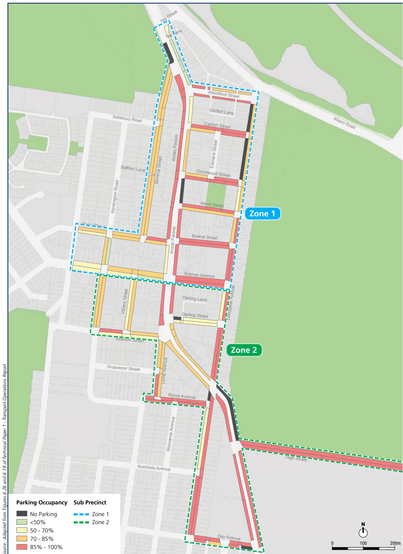
Figure 16.4 Average interpeak (10 am–2 pm) parking occupancy and parking survey zones – Kensington sub-precinct
