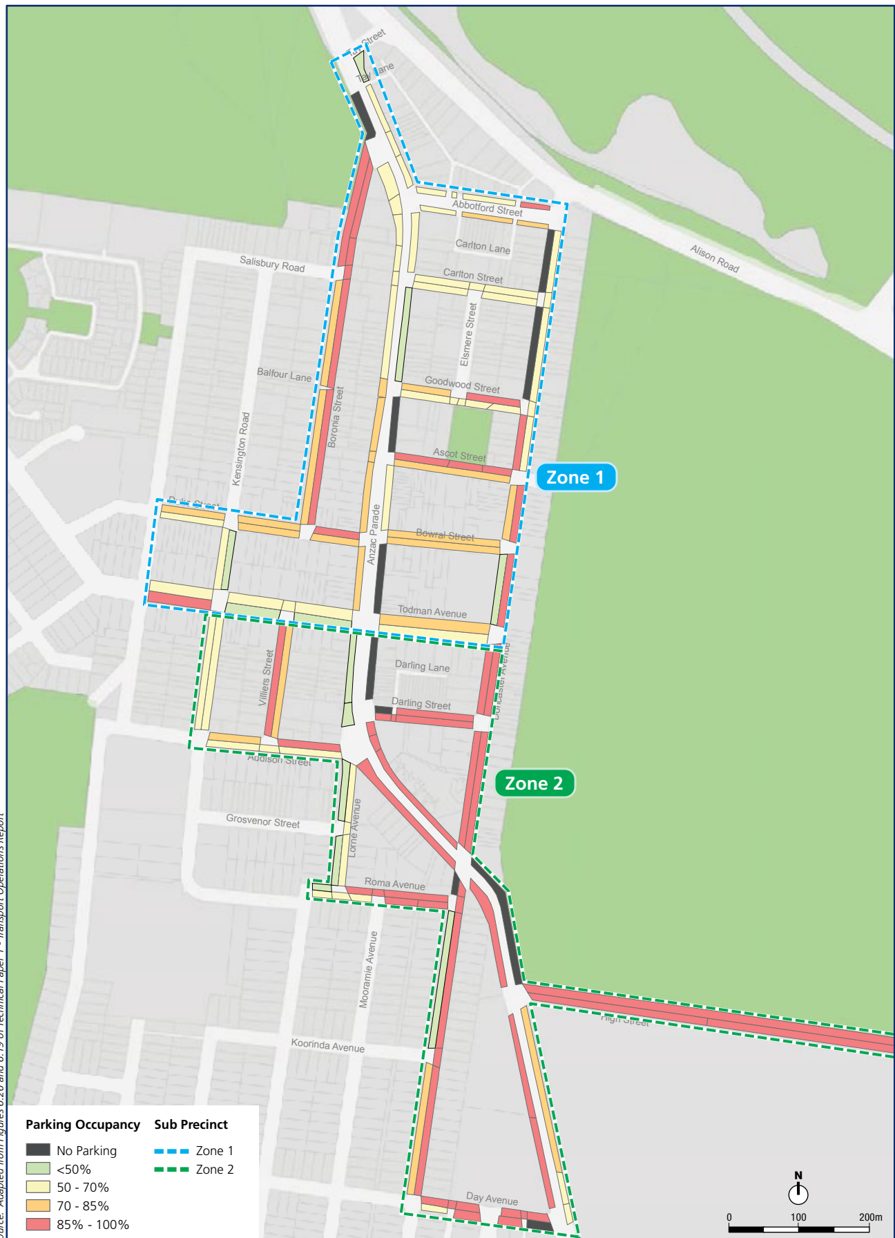
Figure 16.5 Average post-afternoon peak (after 6.30 pm) parking occupancy and parking survey zones – Kensington sub-precinct
