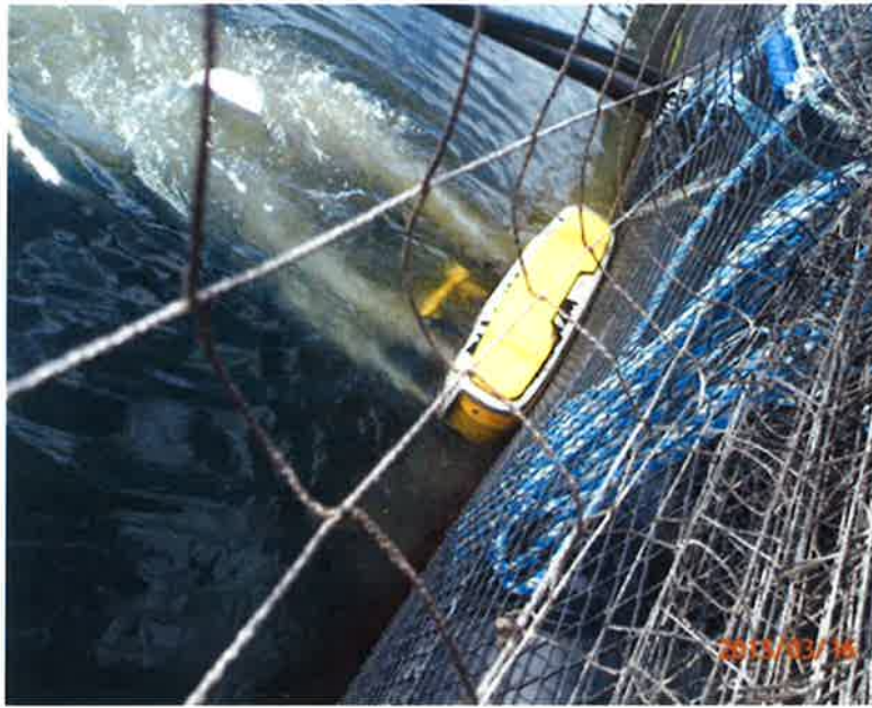
Figure 5: Proposed in situ net cleaner
