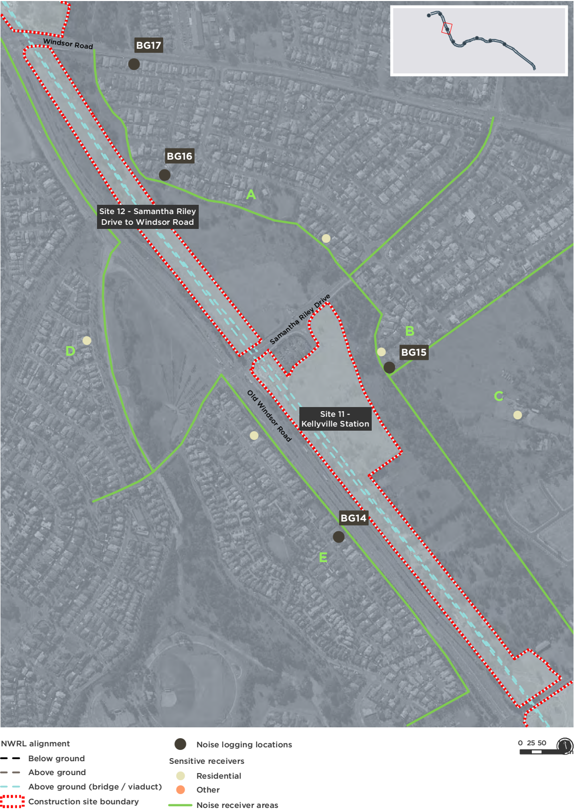
Figure 10.9 Location of sensitive receivers near Kellyville Station
