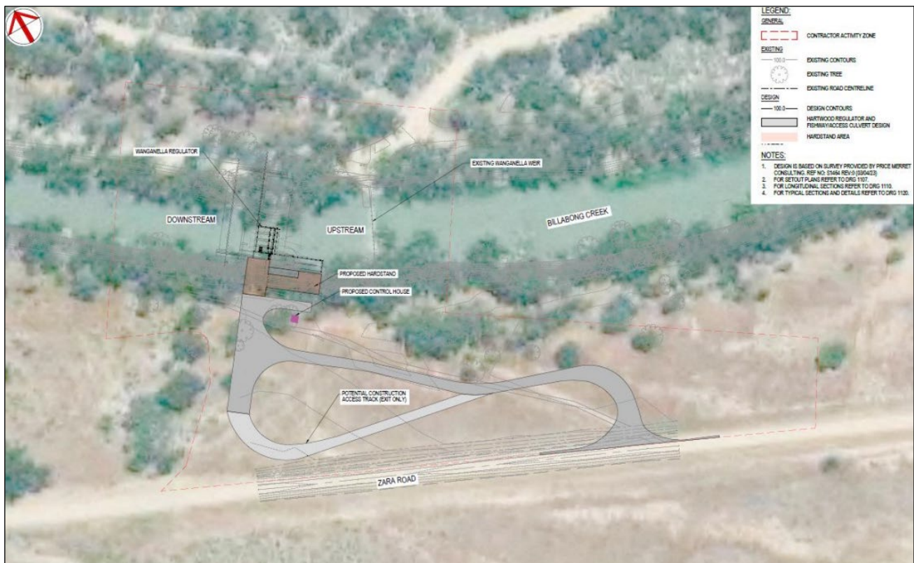
Figure 9 | Indicative Wanganella Regulator layout (Source: EIS)
