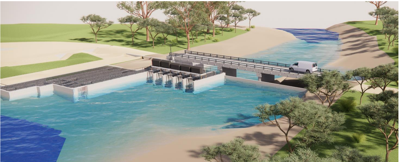
Figure 1.2 Indicative layout of a regulator
