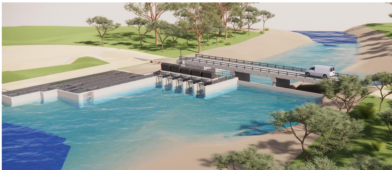
Figure 1.2 Indicative layout of a regulator
