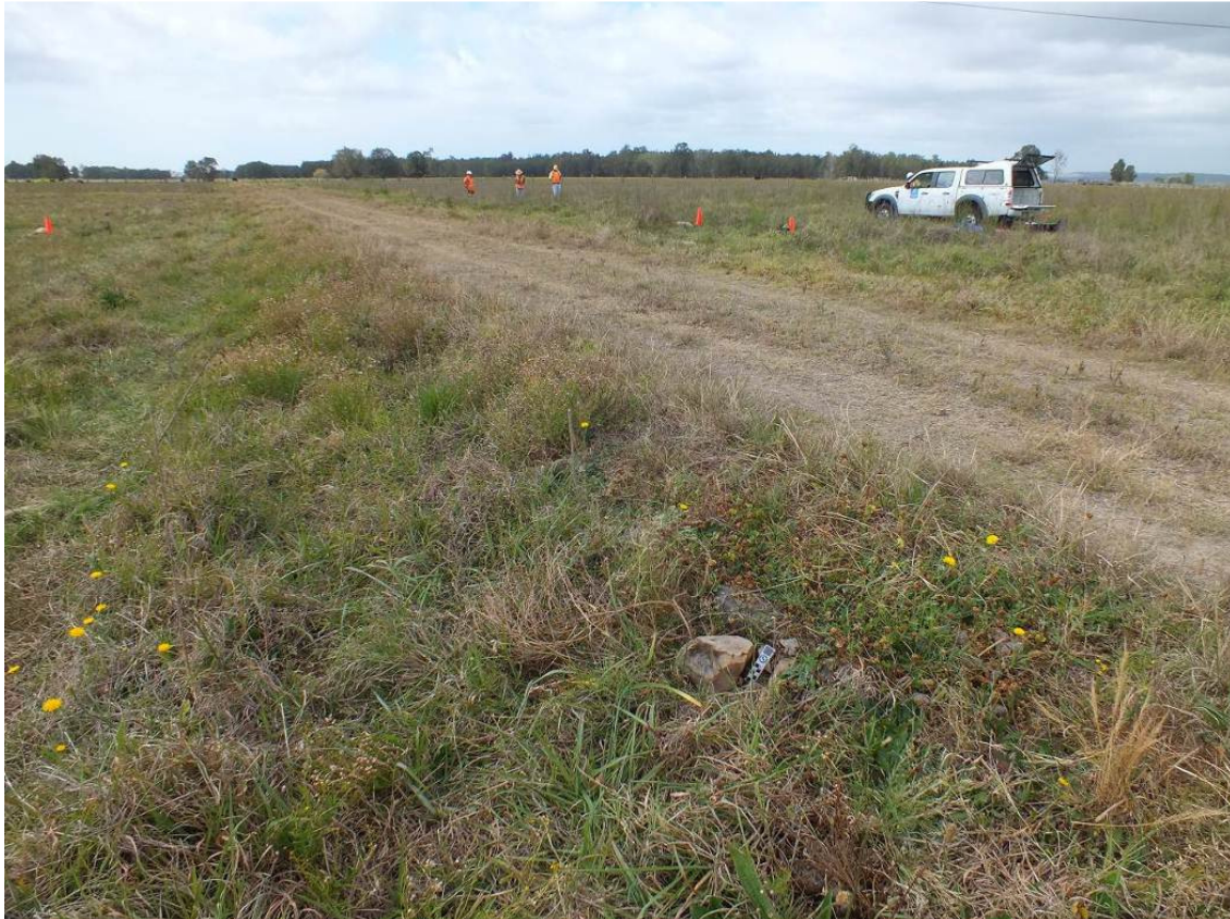
Figure 6.4 IMTC stone core on edge of disused access track (view to south-east).
