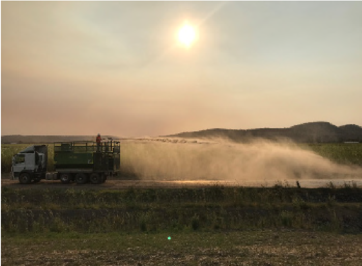
Figure 60 A water cart in Section 5 reusing water for dust suppression
