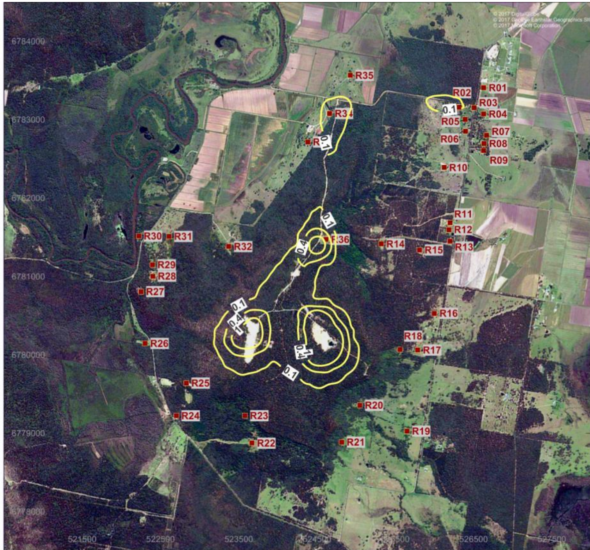
Figure C 6 Predicted incremental annual average dust deposition rate (g/m 2 /month) – proposed year 2 operations
