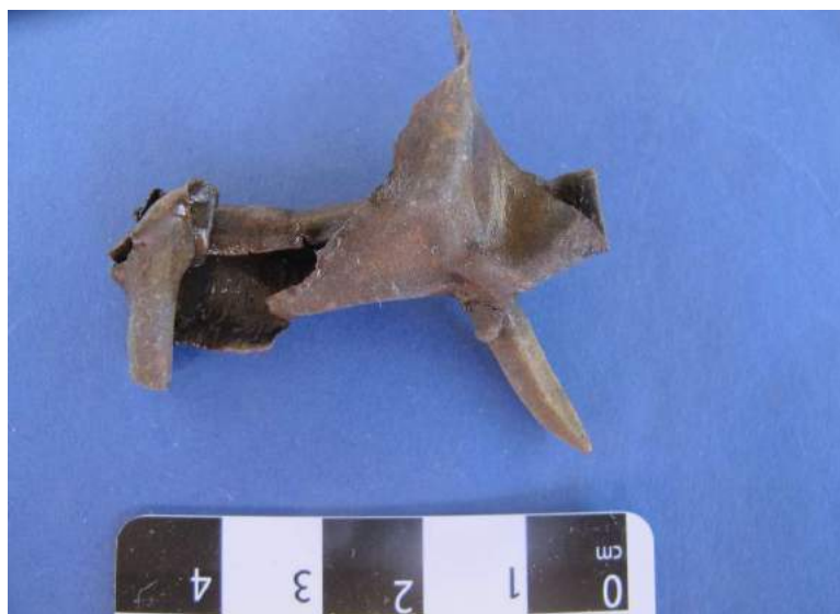
Figure 284 Copper alloy sheathing fragment with copper alloy nail embedded. This artefact given its context could be associated with a vessel as opposed to the 1862 Wharf however an analysis of the chemical composition of the copper alloy may be required. Artefact ID 3385, DT 1, Sq 1, Cxt 06.
