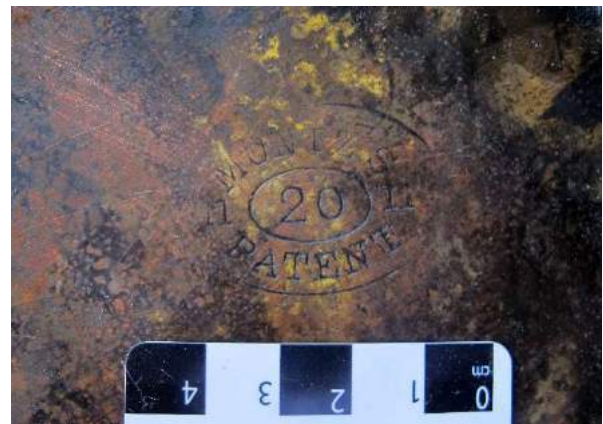
Figure 154: Muntz Metal sheathing; stamp (detail on right) reads “MUNTZ PATENT 11 20 11” (DT1/SQ6/C05).
