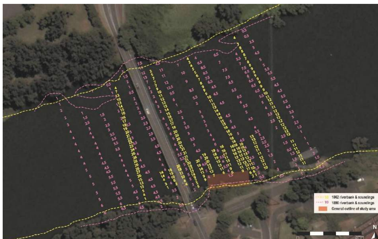
Figure 10: Riverbank outline and depth soundings taking during 1862 and 1890 hydrographic surveys of the Hawkesbury River at Windsor – soundings are shown in feet and reduced to low water Spring tides – overlain on 2019 aerial photograph.
