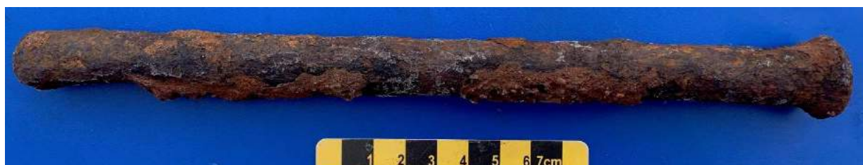
Figure 148: Dump or bolt hammered at both ends. 242 mm long and 15 mm diameter was possibly a keel bolt for a boat or a frame bolt for a larger vessel (T3 / C04 / Spit 2).
