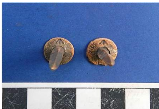
Figure 147: Square wrought copper alloy nails with applied heads that bear the British Government property broad arrow stamp on the underside of the heads (DT2 / C15).
