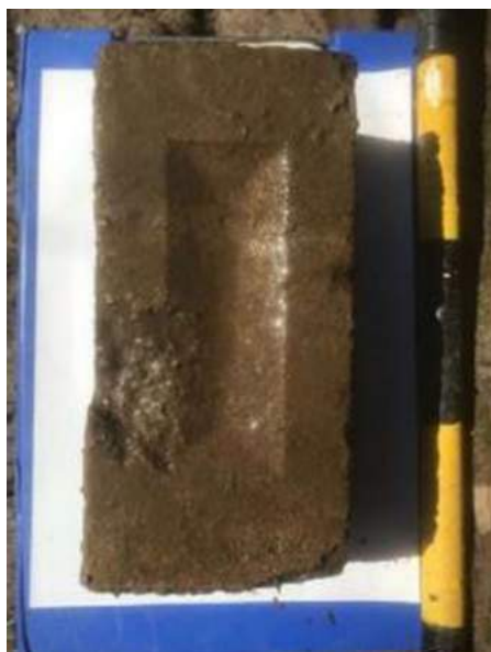
Figure 124: Dry, pressed shale brick. Scale in 100 mm increments.
