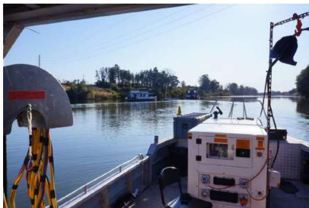
Figure 84: View to the bow of the Dive Boat; (showing from left to right), diver umbilical and 33 KVA electrical generator for the pump.
