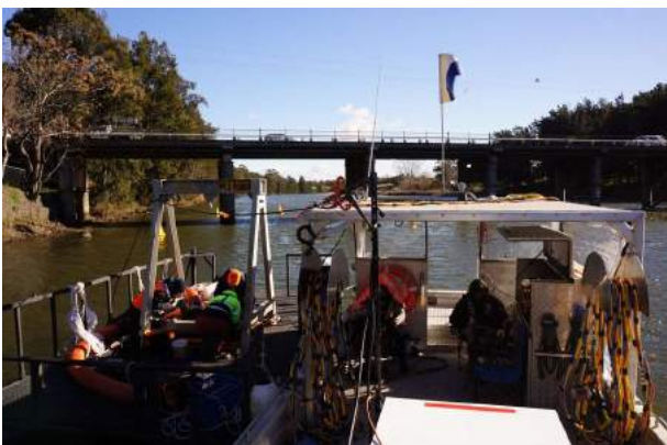
Figure 83: View to the stern of the Dive boat; (showing from left to right), barge, dive boat with SSBA dive panel, diver umbilicals, tools and generator in bottom right corner.
