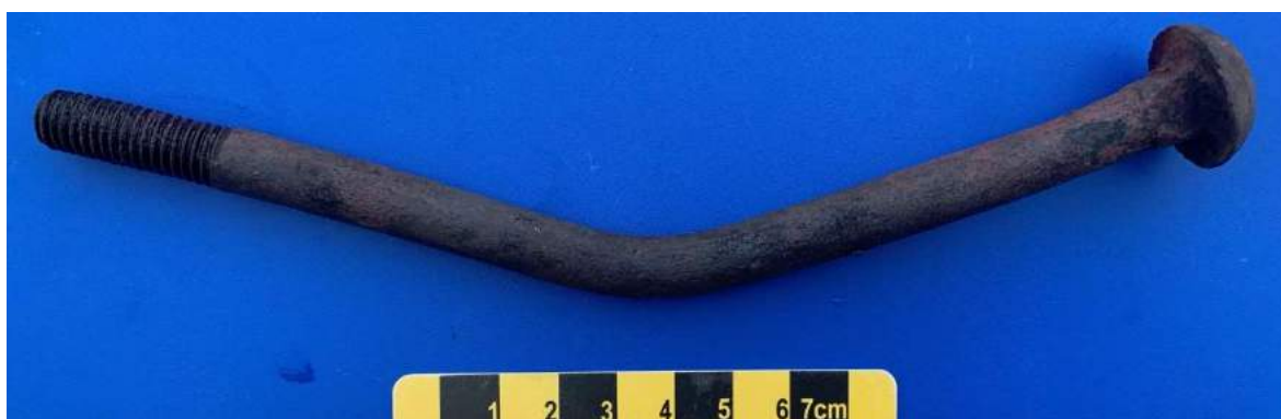
Figure 274: Threaded through bolt, 11 mm diameter and 180 mm long. Artefact ID 5279, ST 1, Cxt 04.
