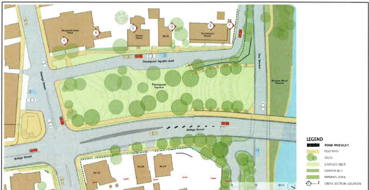
Figure 7: Future new road configuration in Thompson Square
