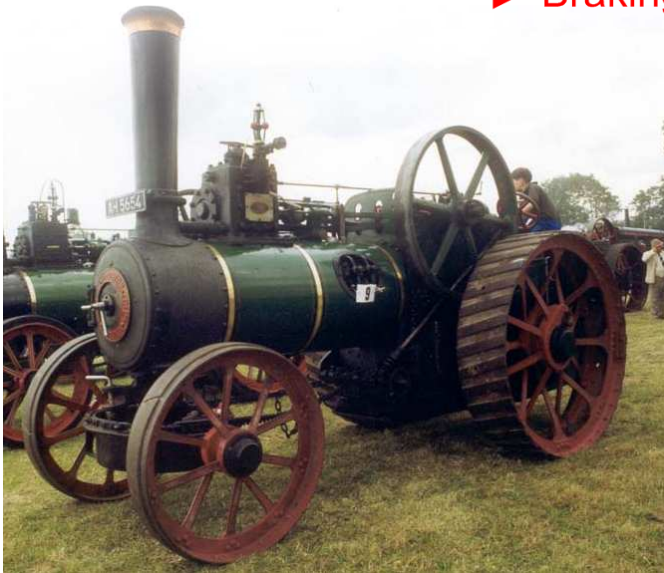
1908 Ruston Proctor Traction Engine – 9.5t
