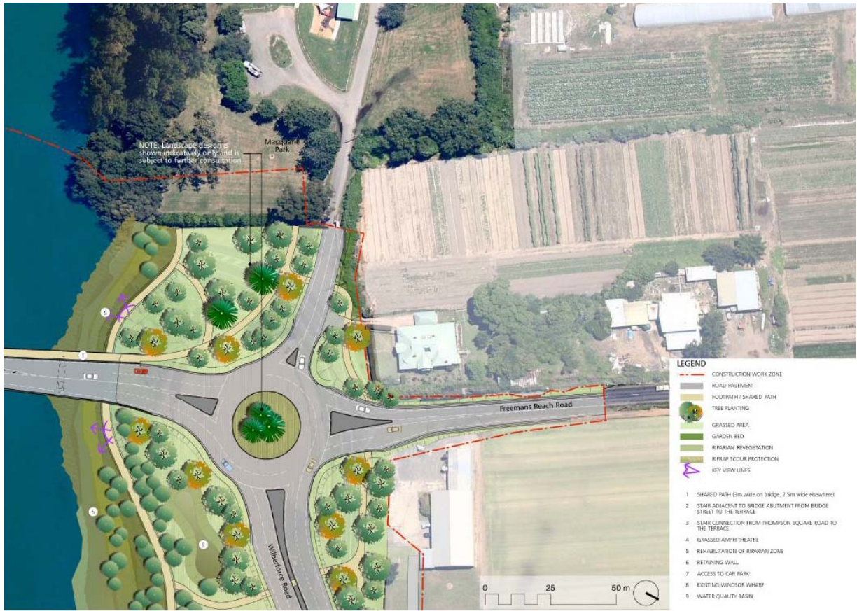
Plate 122: Detail from the landscape concept plan prepared by Spackman Mossop and Michaels with Hills Thallis; page 77. The northern bank would be landscaped with a combination of grass, trees, a riparian zone to screen the scour protection and the roundabout.
