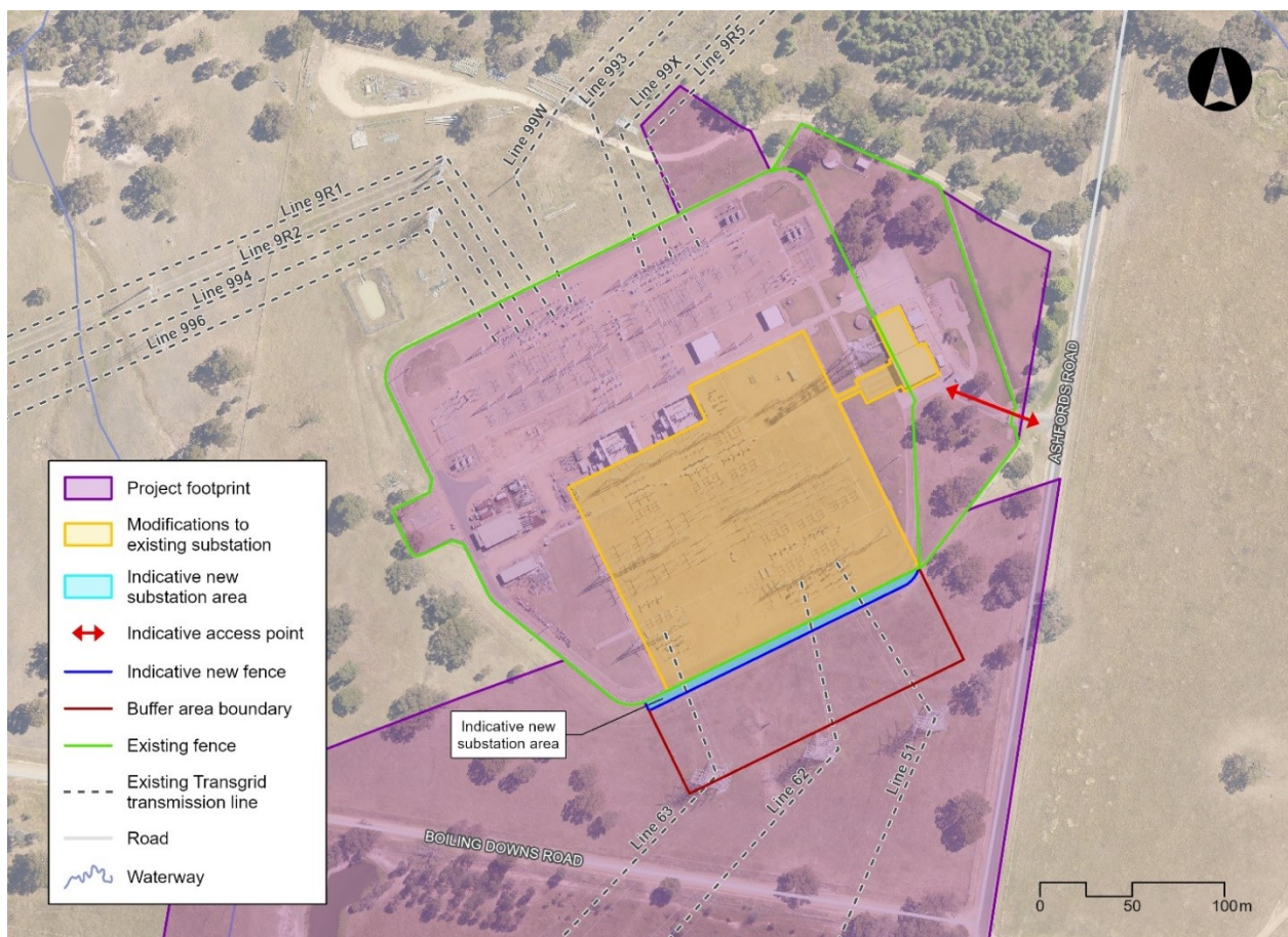
Figure 7-2 Indicative layout of modified Wagga 330 kV substation showing location of the existing access from Ashfords Road
