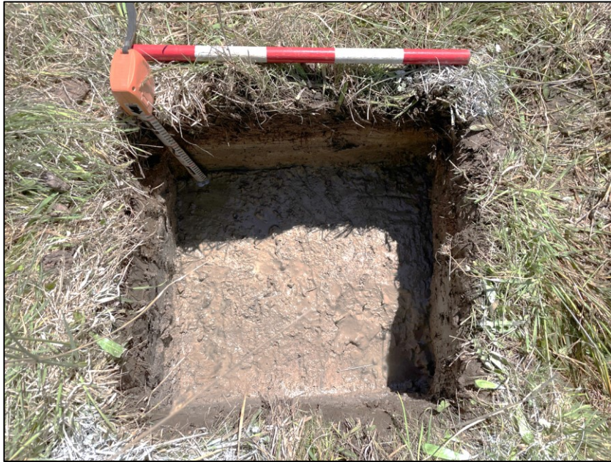
Figure 8-29 PAD-10 Test Pit 7 showing evidence of water seepage from the water table
