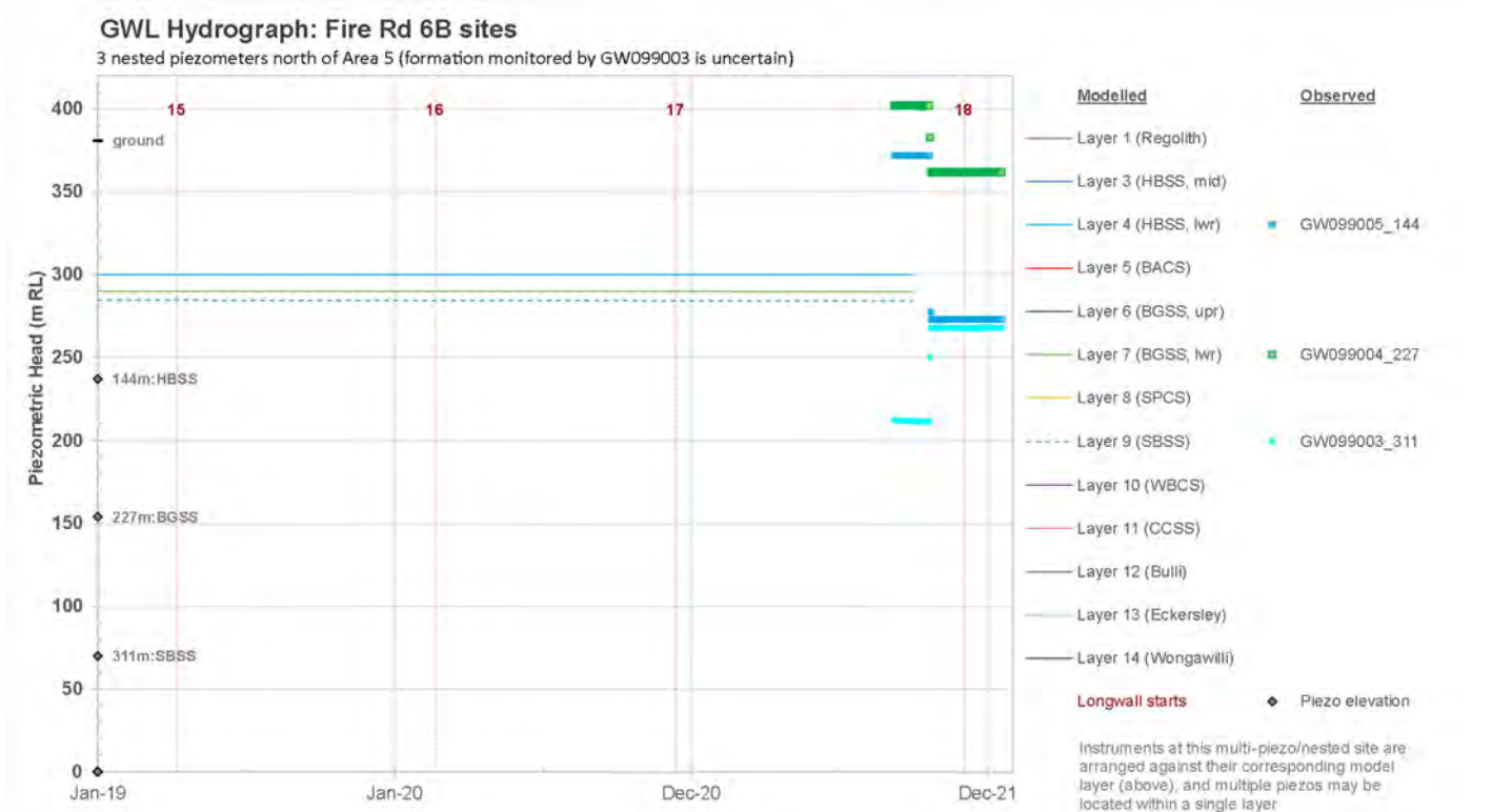
Figure 5-12 Modelled vs observed groundwater level at DPIE-W bores – Fire Trail 6B
