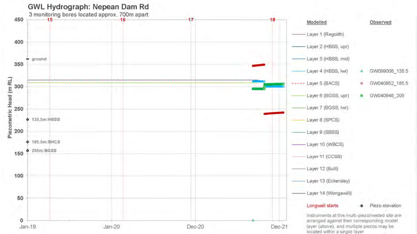
Figure 5-11 Modelled vs observed groundwater level at DPIE-W bores – Nepean Dam Rd
