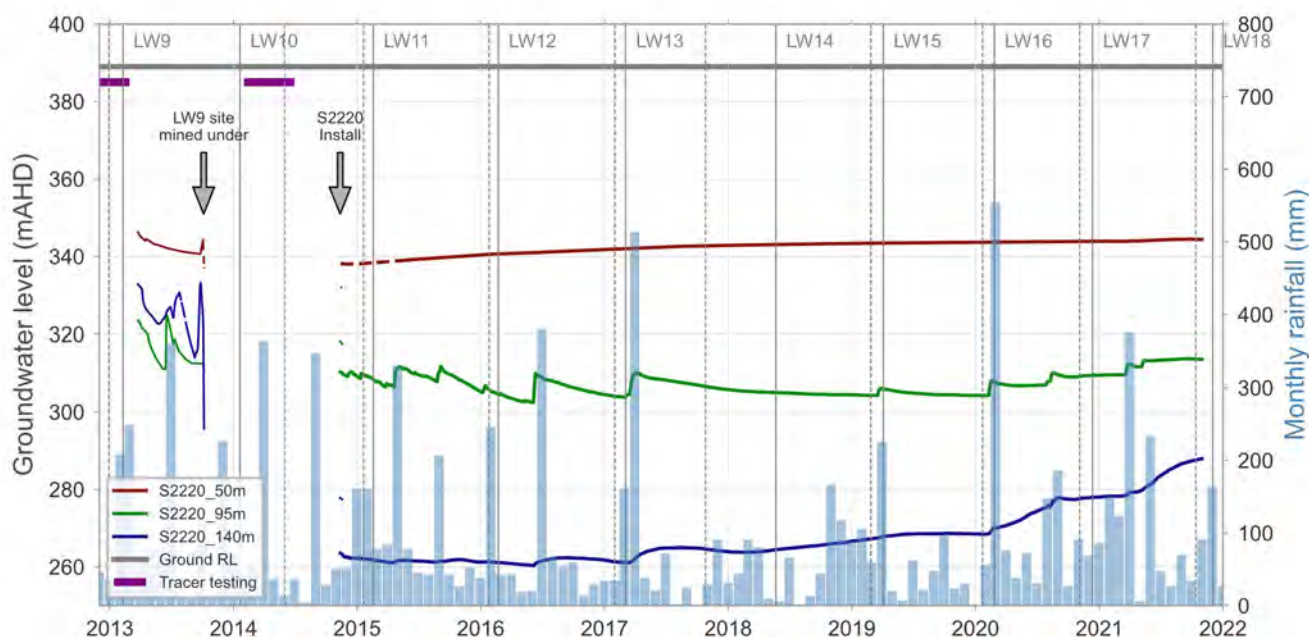
Figure 2-16 Groundwater level trends above a longwall (Longwall 9, bores S2192-S2220)
