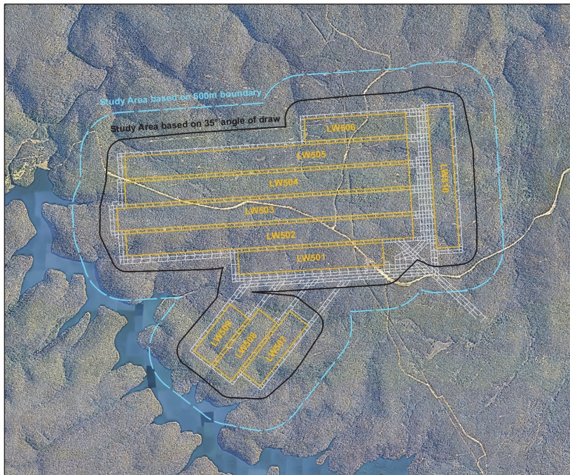
Fig. 1.2 Aerial photograph showing the proposed longwalls and the Study Area
