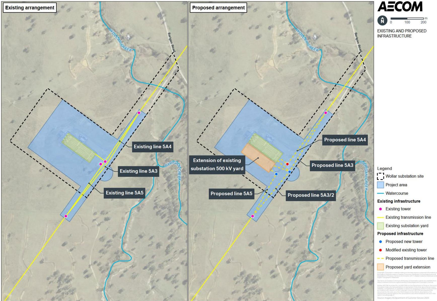
Figure 3-2 Key components of the Wollar Substation Upgrade project
