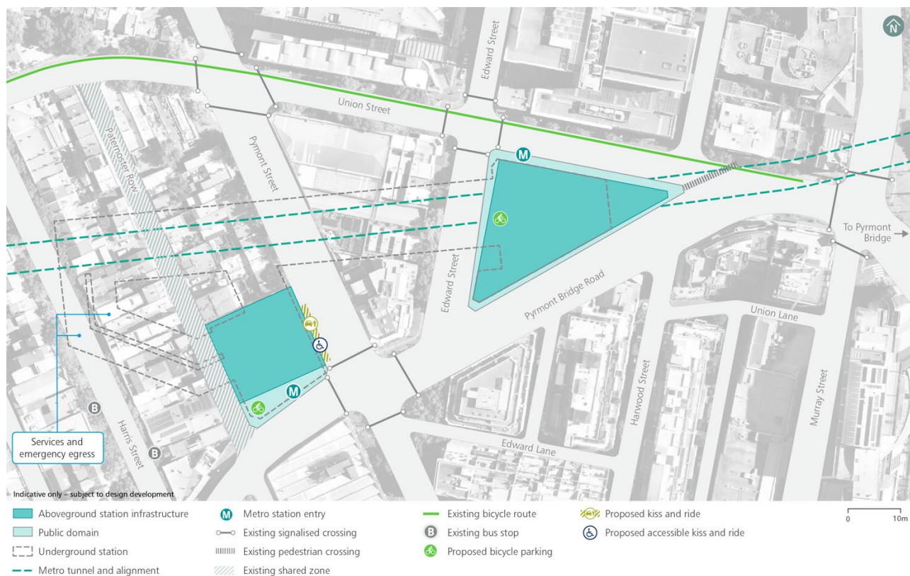
Figure 11-2 Pyrmont Station indicative layout and key design features
