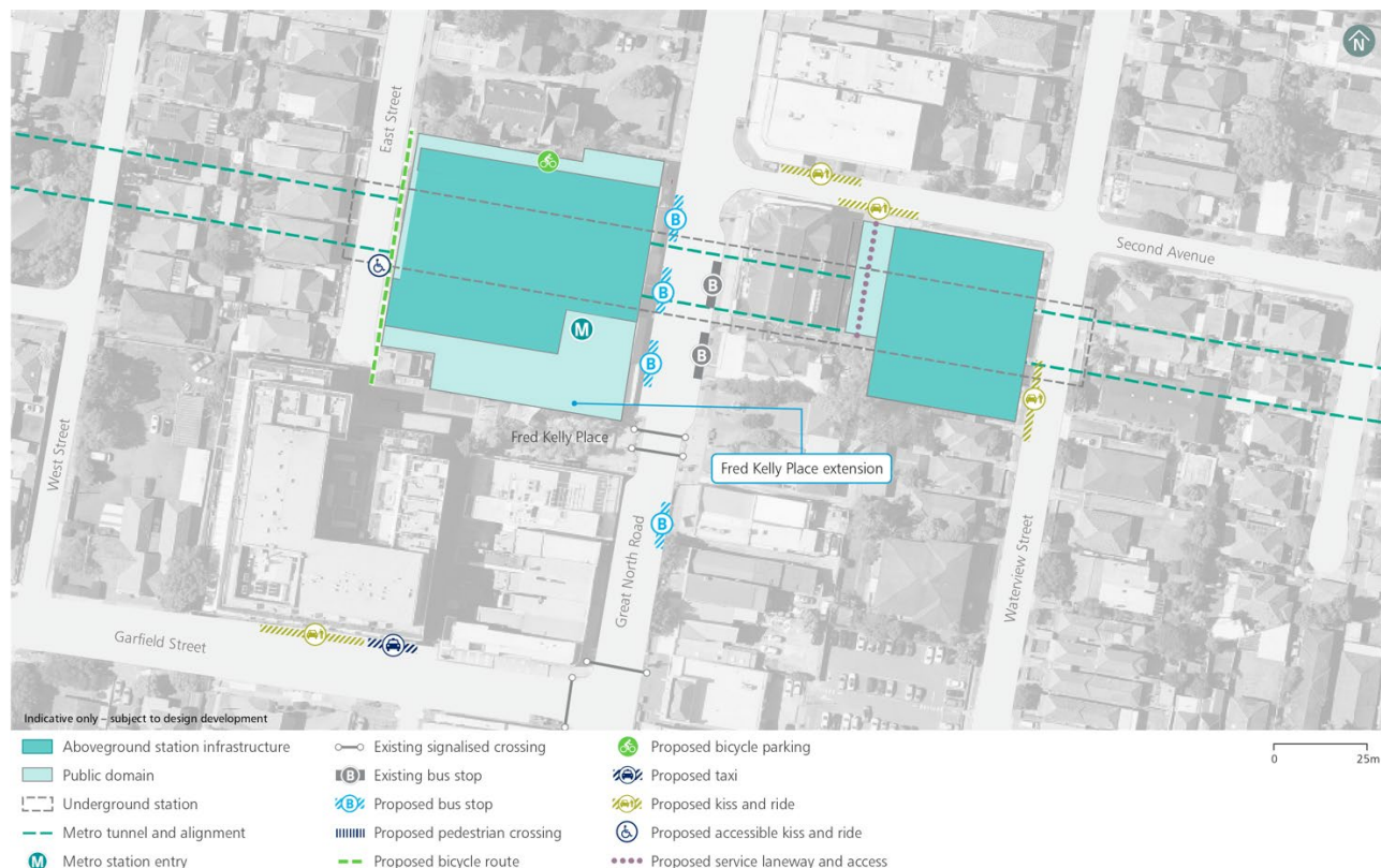
Figure 9-2 Five Dock Station indicative layout and key design elements
