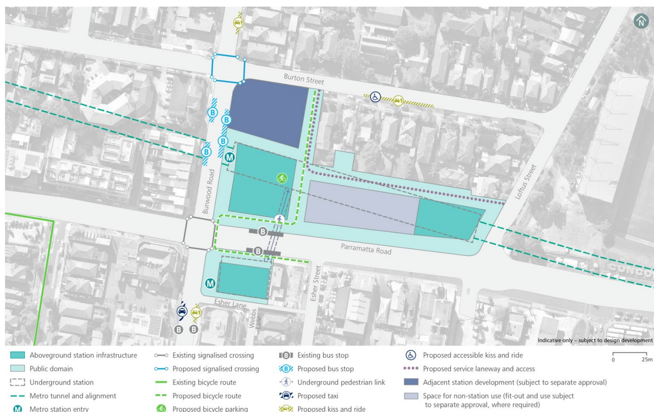
Figure 8-2 Burwood North station indicative layout and key design elements
