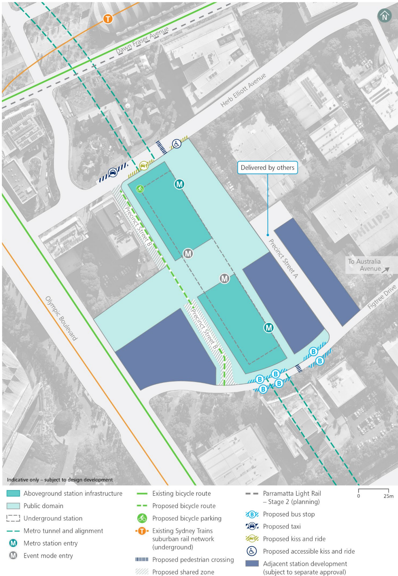
Figure 6-2 Sydney Olympic Park metro station indicative layout and key design elements
