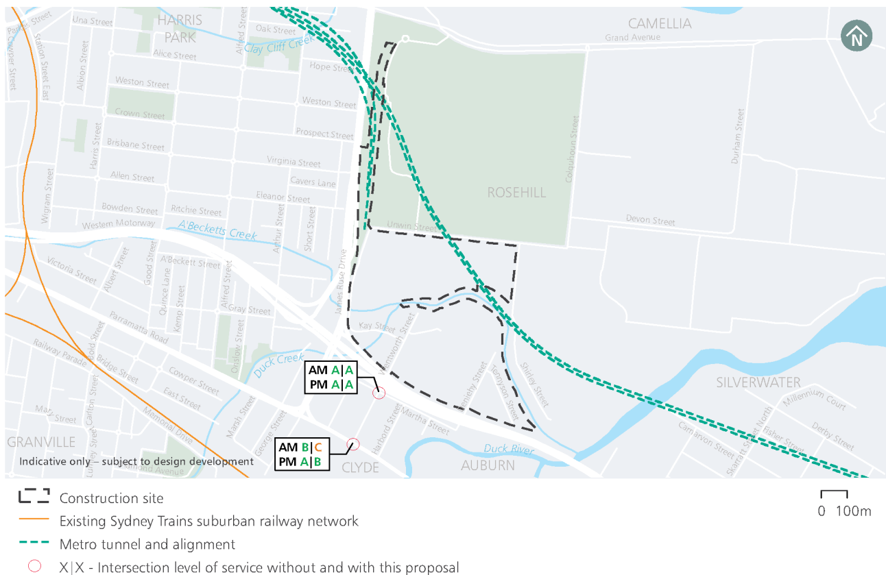
Figure 17-9 Construction site intersection performance – Clyde stabling and maintenance facility and Rosehill services facility (2026)
