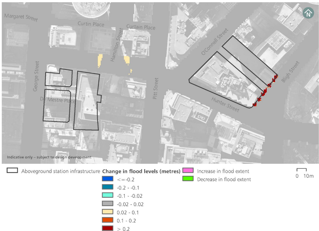
Figure 15-20 Potential change in flood levels (one per cent AEP event) – Hunter Street Station (Sydney CBD)
