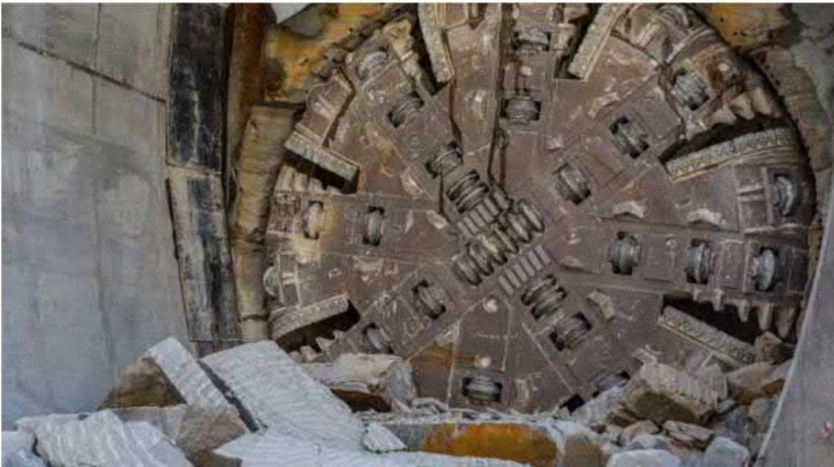
Figure 5-9 Photo of a TBM used to construct the Sydney Metro Northwest Line
