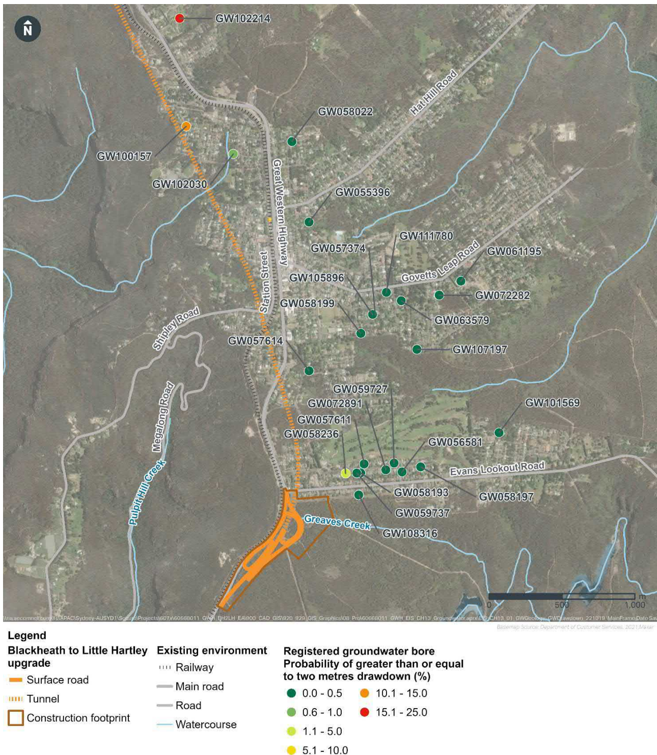
Figure 13-9 Predicted maximum groundwater drawdown (95 th percentile) at registered groundwater bores during construction at Blackheath
