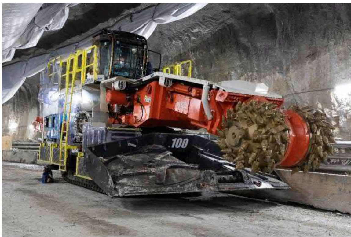
Figure 5-11 Photo of a roadheader used to construct the new M6 tunnels
