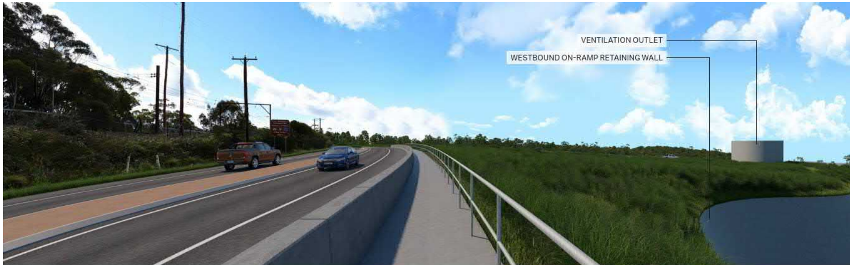
Figure 18-6 Viewpoint 2a – proposed view westbound showing the upgraded Great Western Highway on the left and the ventilation outlet (if selected as the ventilation design) on the right
