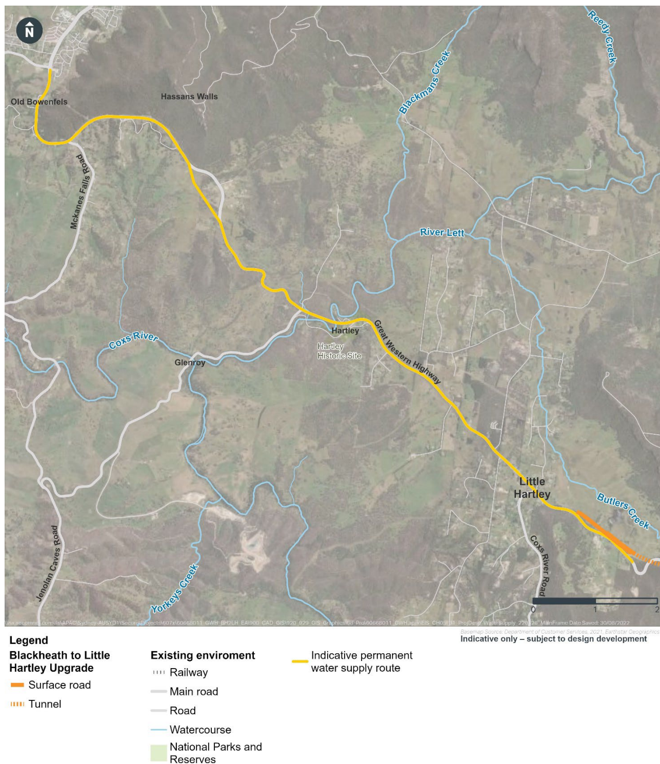
Figure 4-24 Indicative permanent water supply pipeline route
