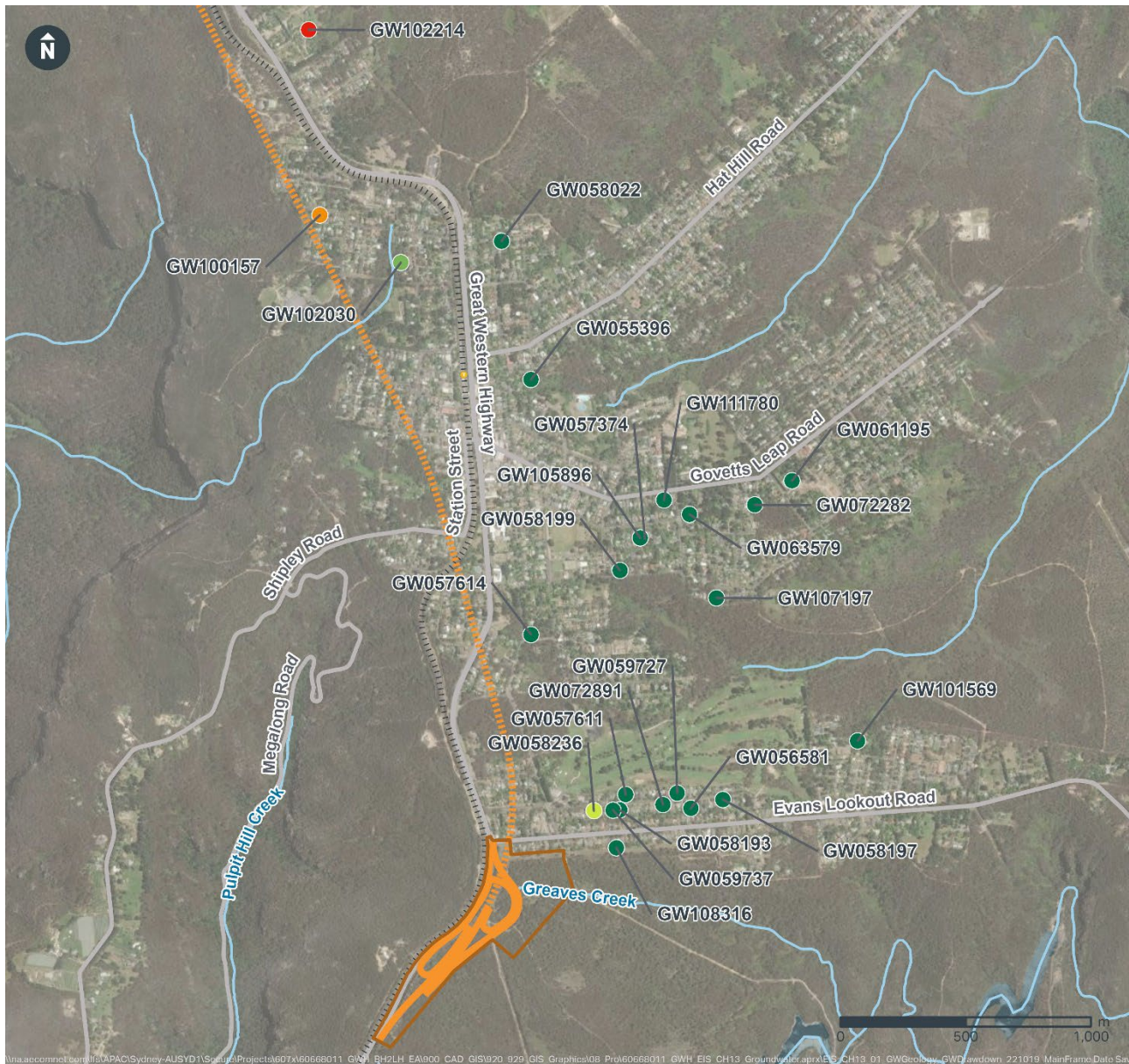
Figure 13-9 Predicted maximum groundwater drawdown (95 th percentile) at registered groundwater bores during construction at Blackheath
