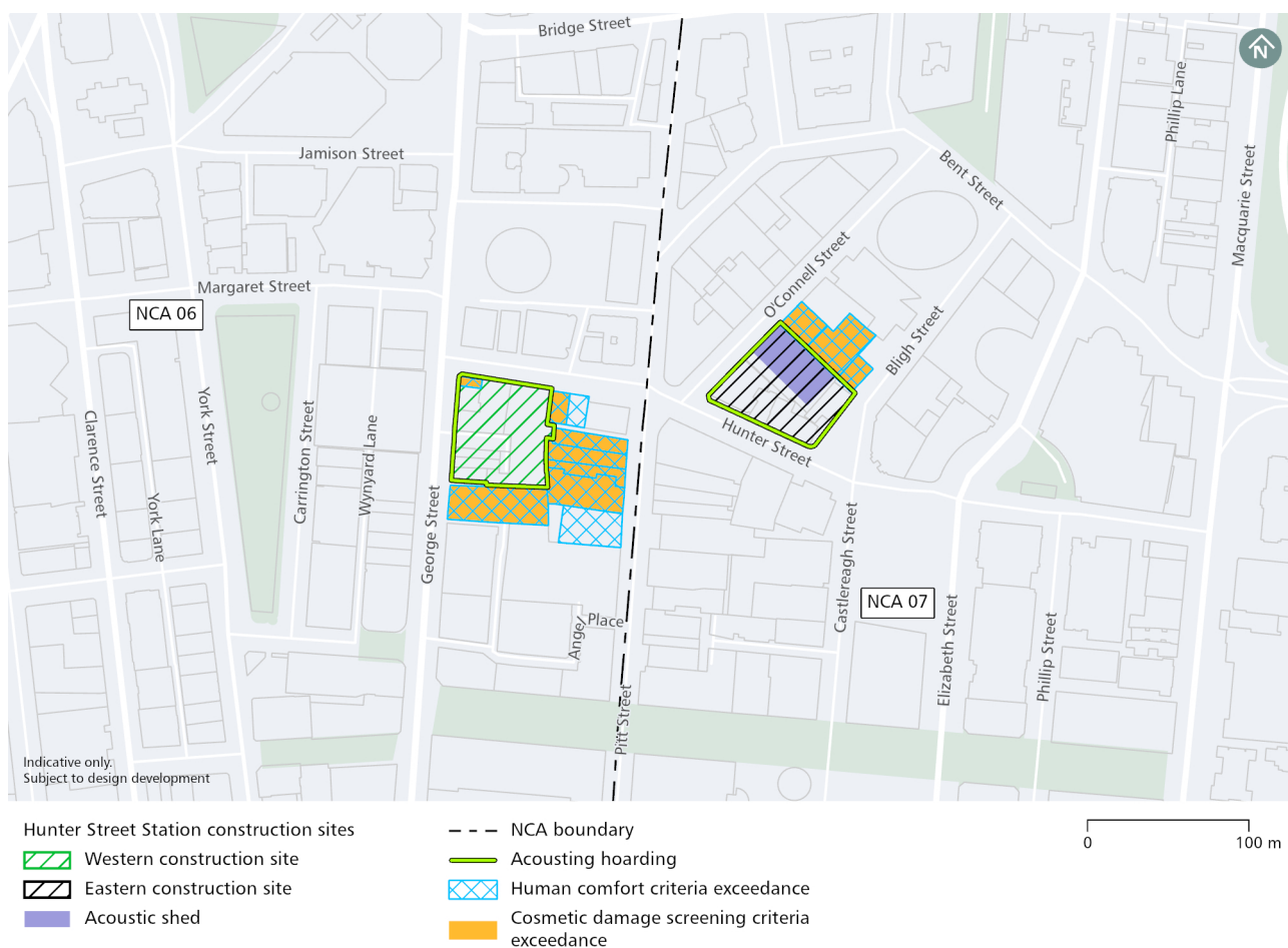
Figure 7-8 Predicted vibration impacts – Hunter Street Station construction site
