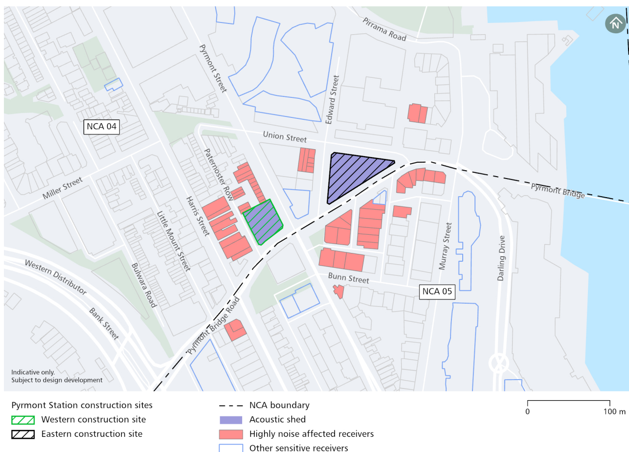
Figure 7-3 Highly noise affected residential receivers - Pymont Station construction sites
