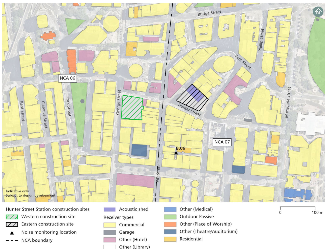
Figure 7-7 Location of sensitive receivers near Hunter Street Station construction sites
