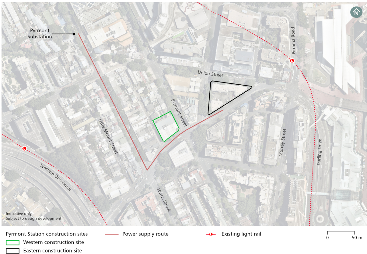
Figure 3-4 Pyrmont Station power supply route
