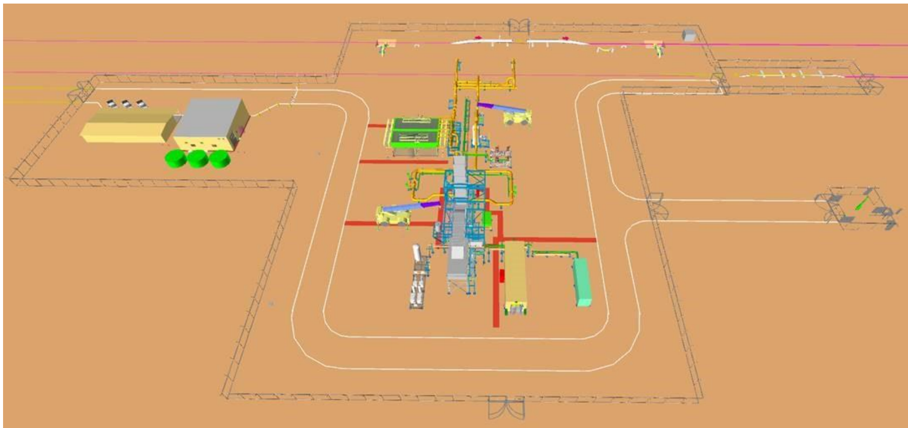
Figure 4.4: Example compression station layout
