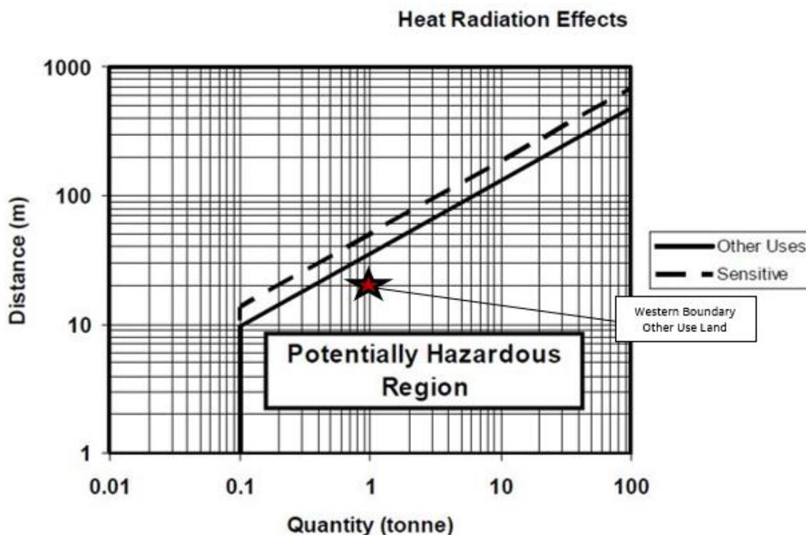
Figure 10.1: Heat radiation effects of gas (after NSW, 2011)
