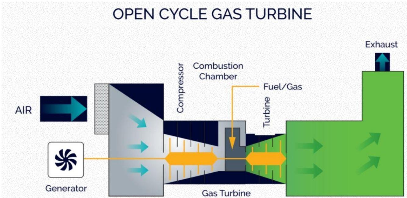
Figure 2.2: Open Cycle Gas Turbine – Schematic diagram
