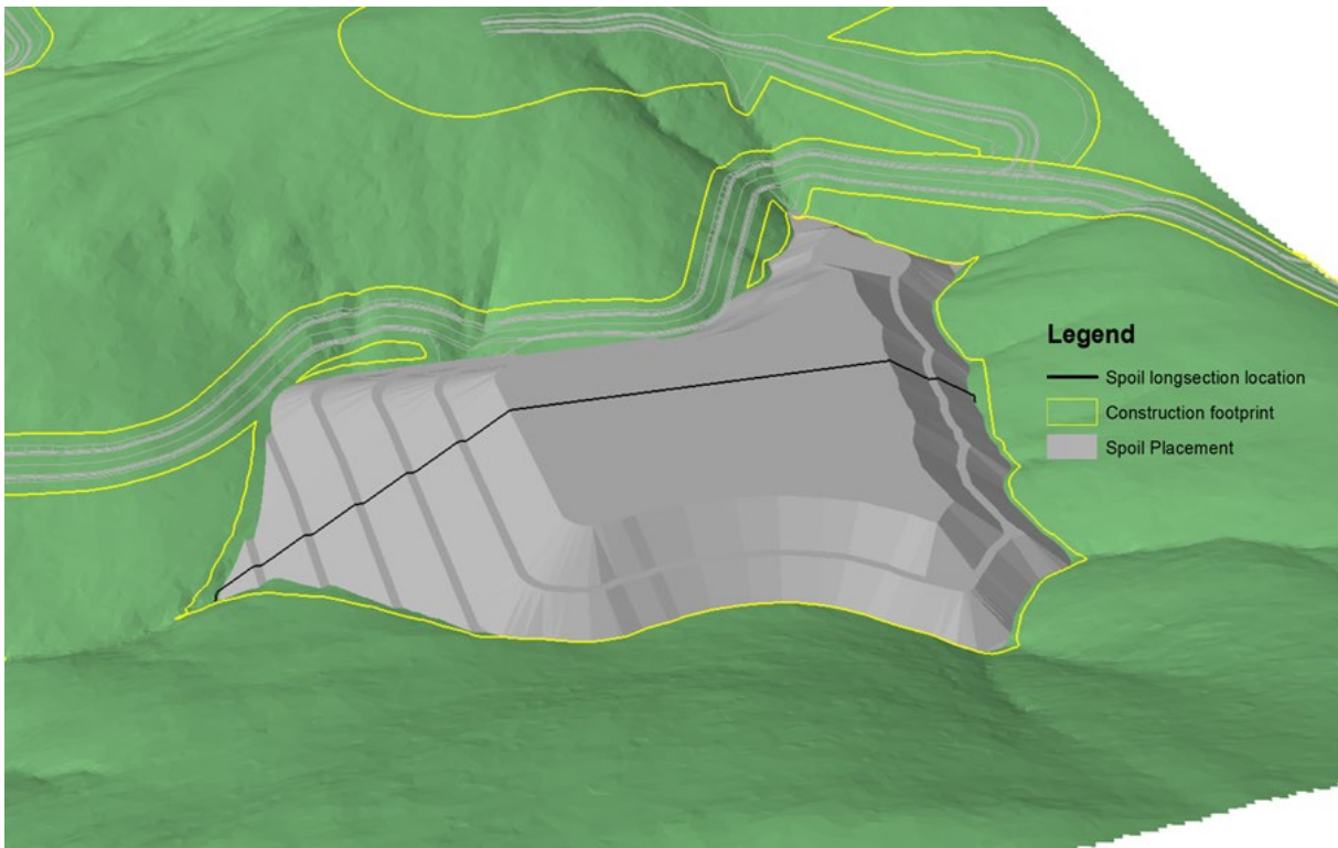
Figure 1.25 Aerial view of lower spoil area B (grey: rockfill, orange: unsuitable)
