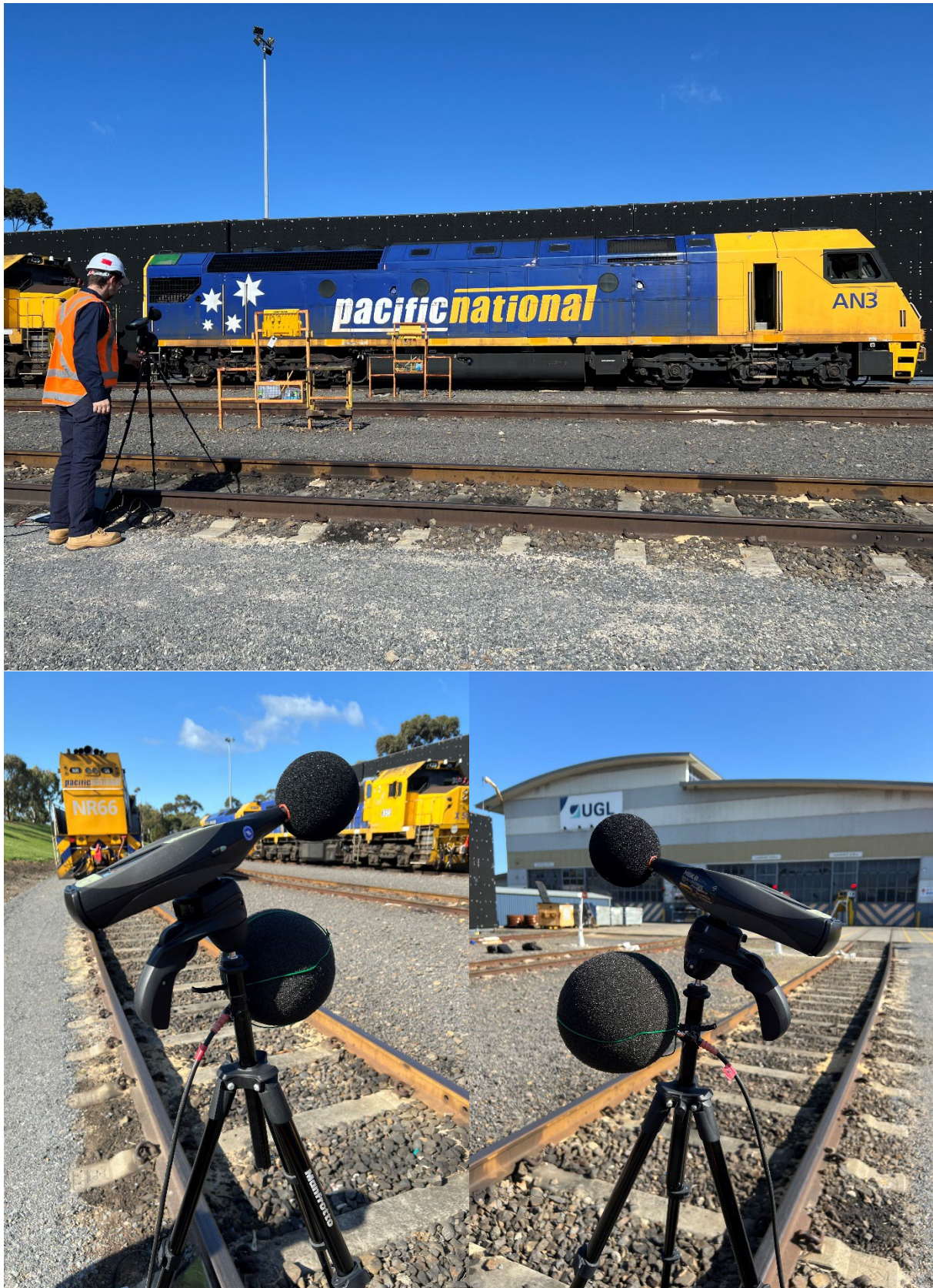
Figure 2 Photos of the noise test location showing the noise barrier and adjacent locomotives (note: also shown is a second microphone which was used as a backup to the sound level meter)
