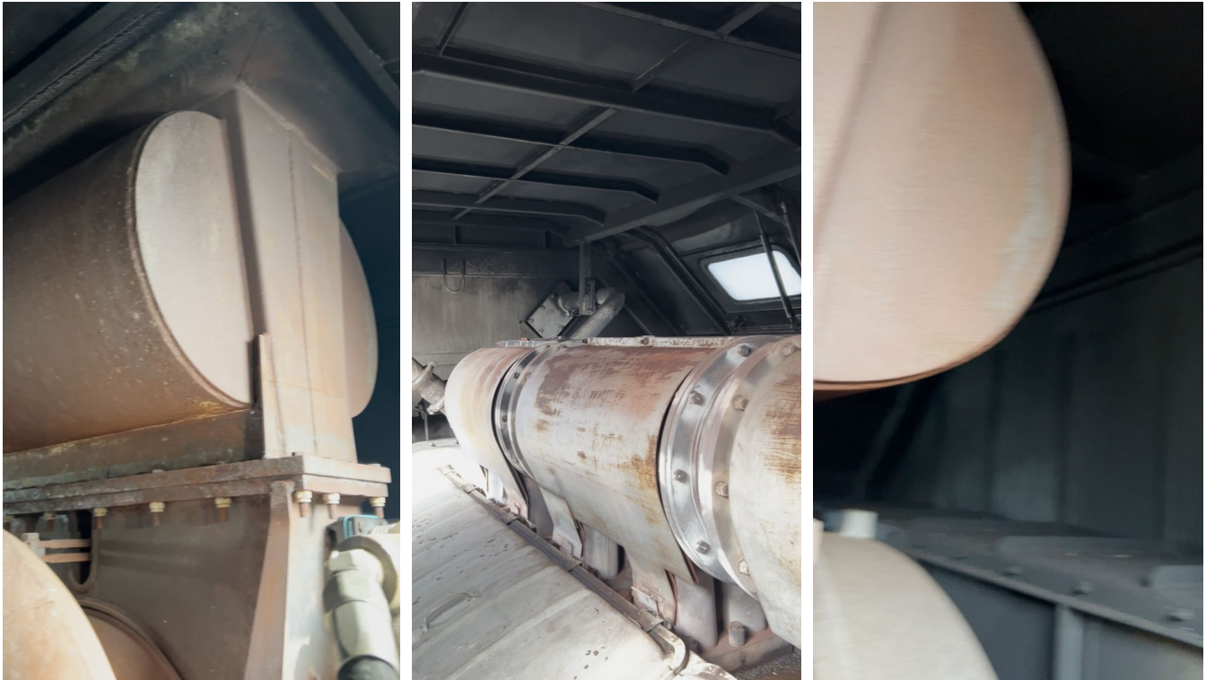
Figure 4 Engine cab photos – existing rudimentary muffler (left), space over the engine manifold (centre) and additional volume above the alternator cab (right) relative to the C Class.
