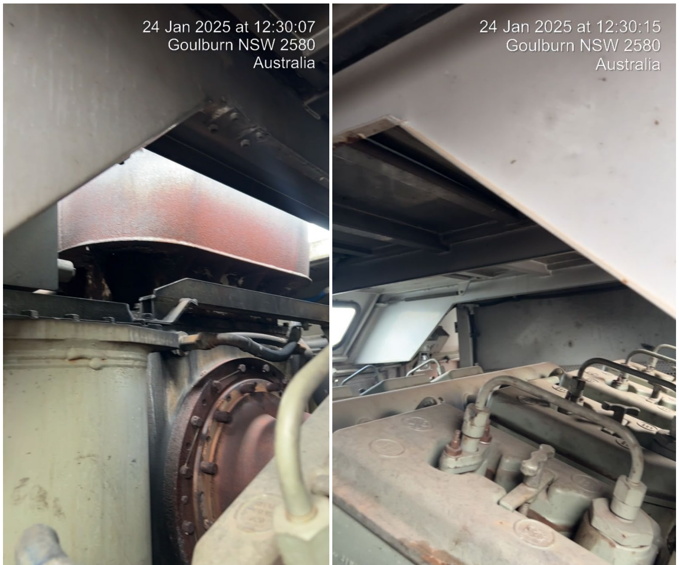
Figure 4 Existing exhaust shaft (left) and empty space above the engine (right) on EL63.
