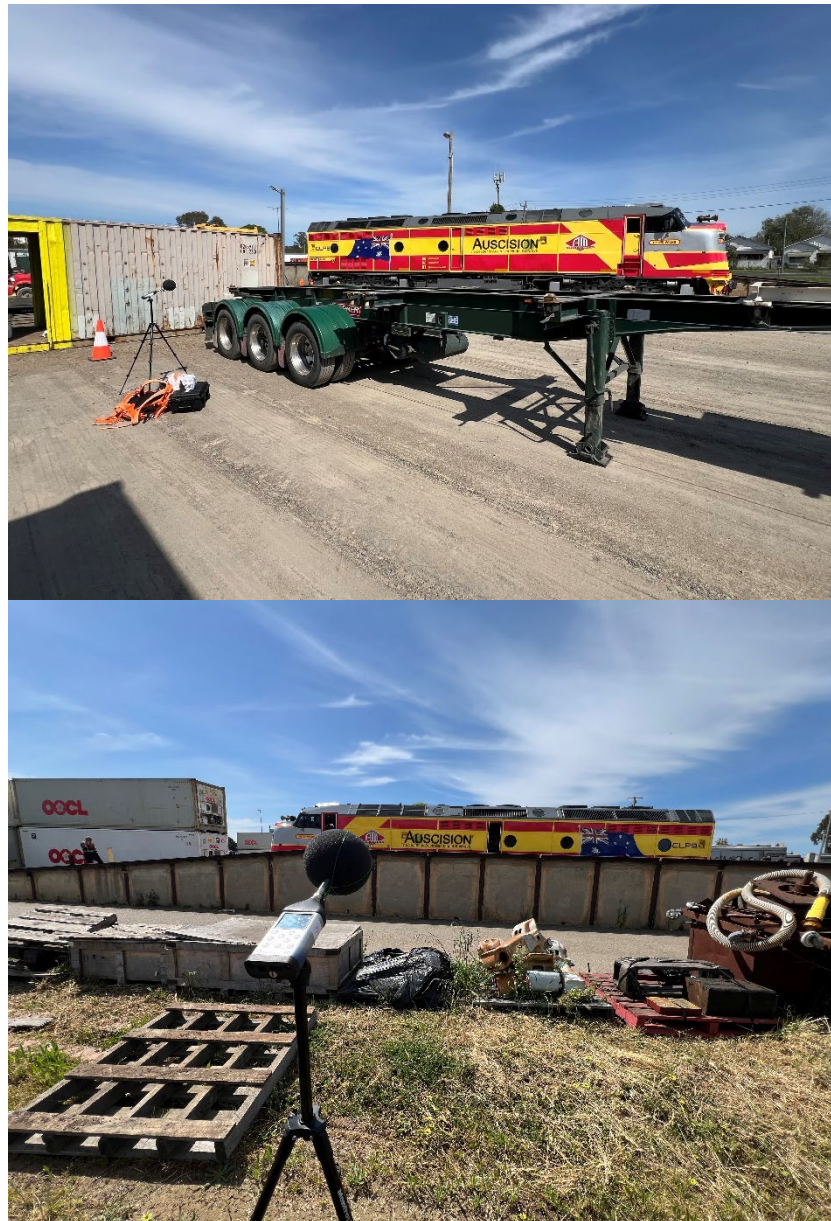
Figure 2 Photos of the noise test location. Note that the engine cab door on the cable side (bottom) was open during the testing. This did not appear to influence the results.
