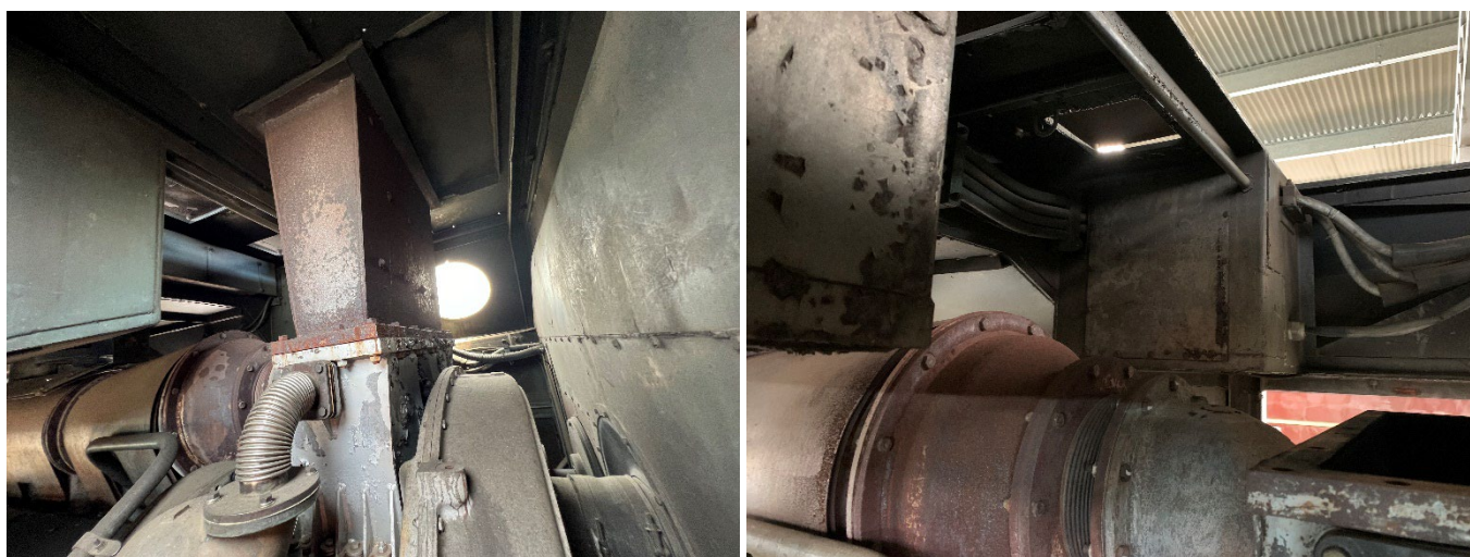
Figure 4 Comparison of the space above the turbocharger in the engine cabs of CLP09 (left) and a C Class (right) locomotive. Note: the exhaust shaft was removed from the C Class but was identical to that in CLP09. Neither the C Class nor CL Class locomotives have mufflers.
