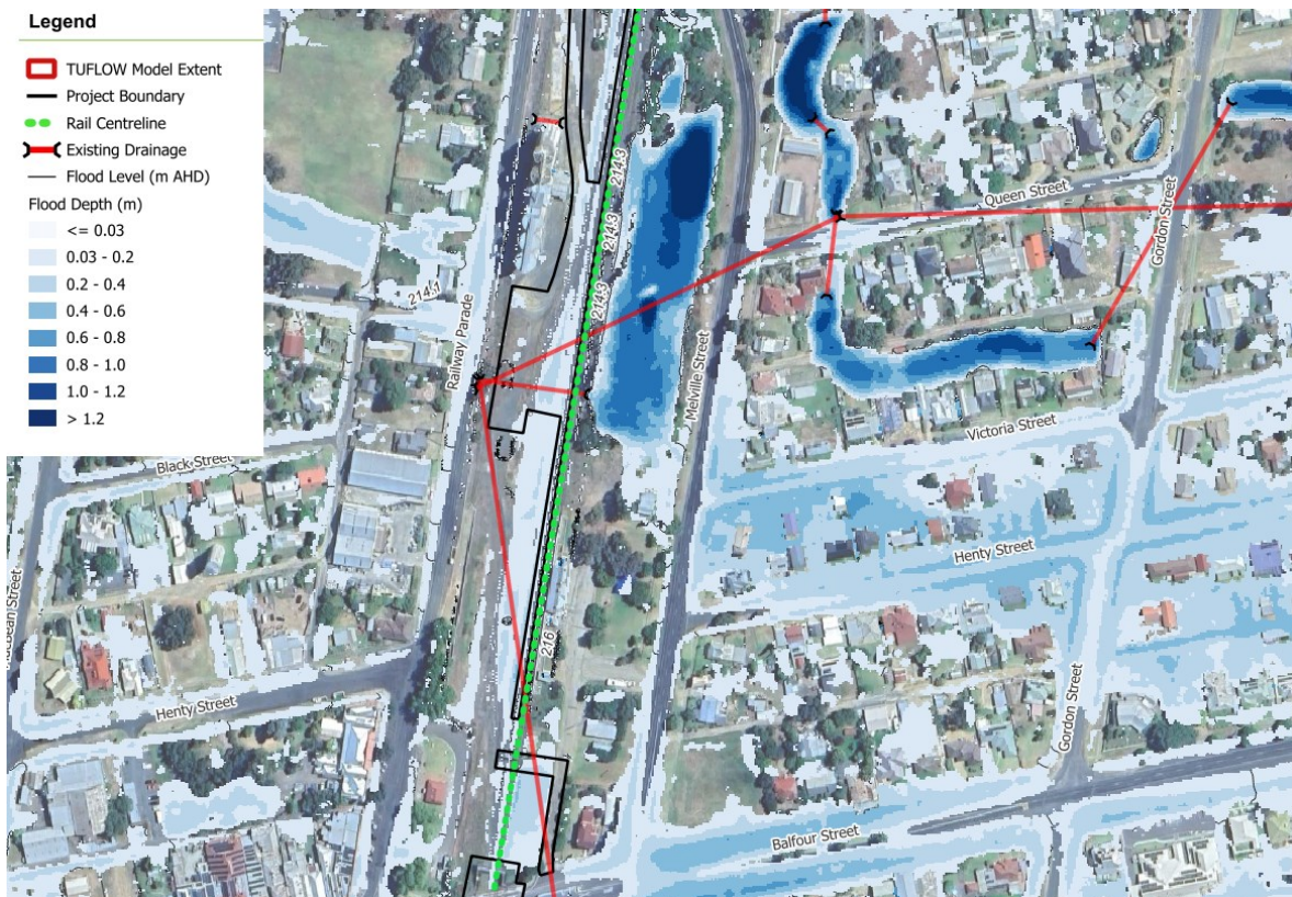
Figure 7-1: 1% AEP Climate Change – Existing Conditions Flood Depth
