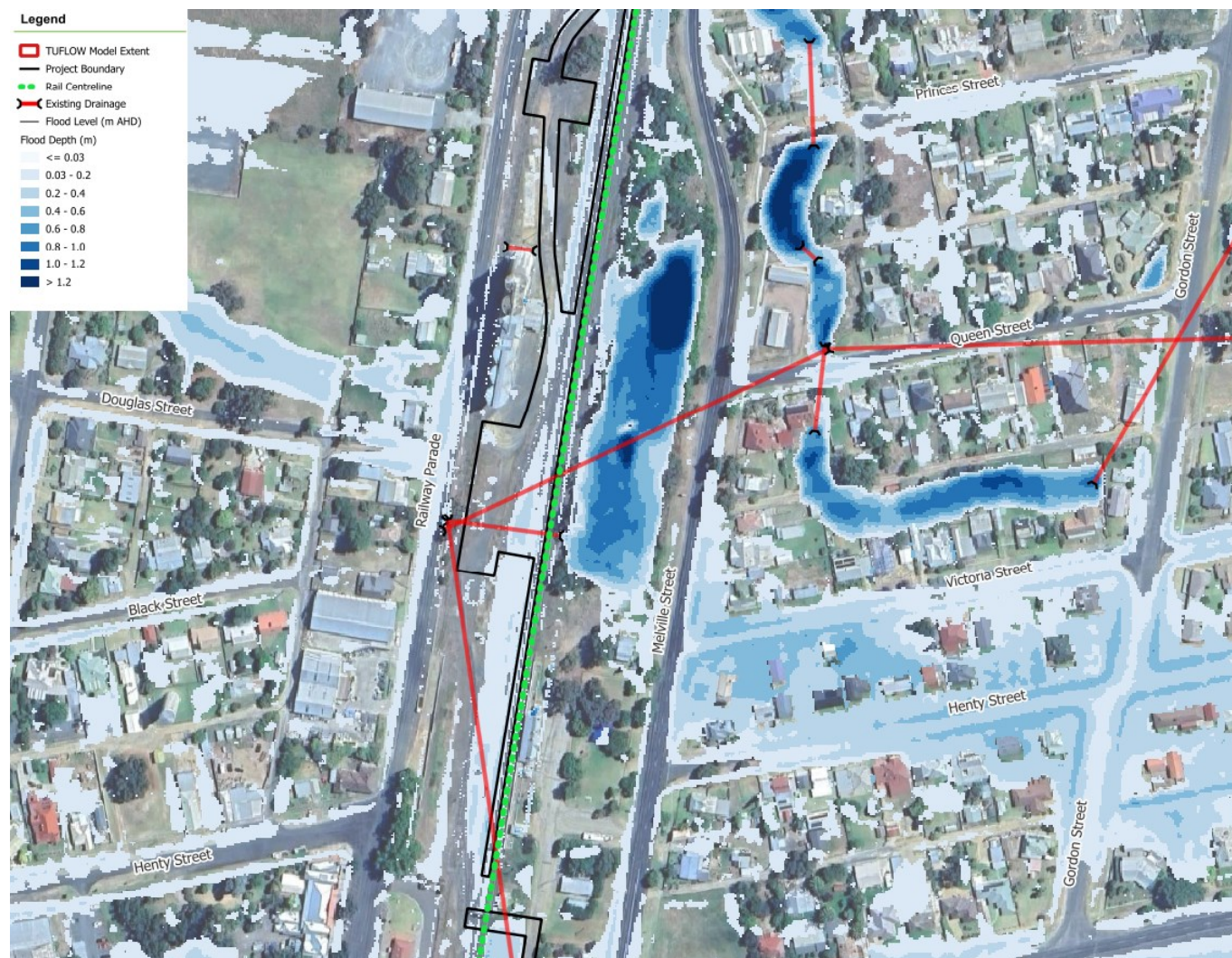
Figure 6-4: Design Conditions Flood Extent – 1% AEP Event
