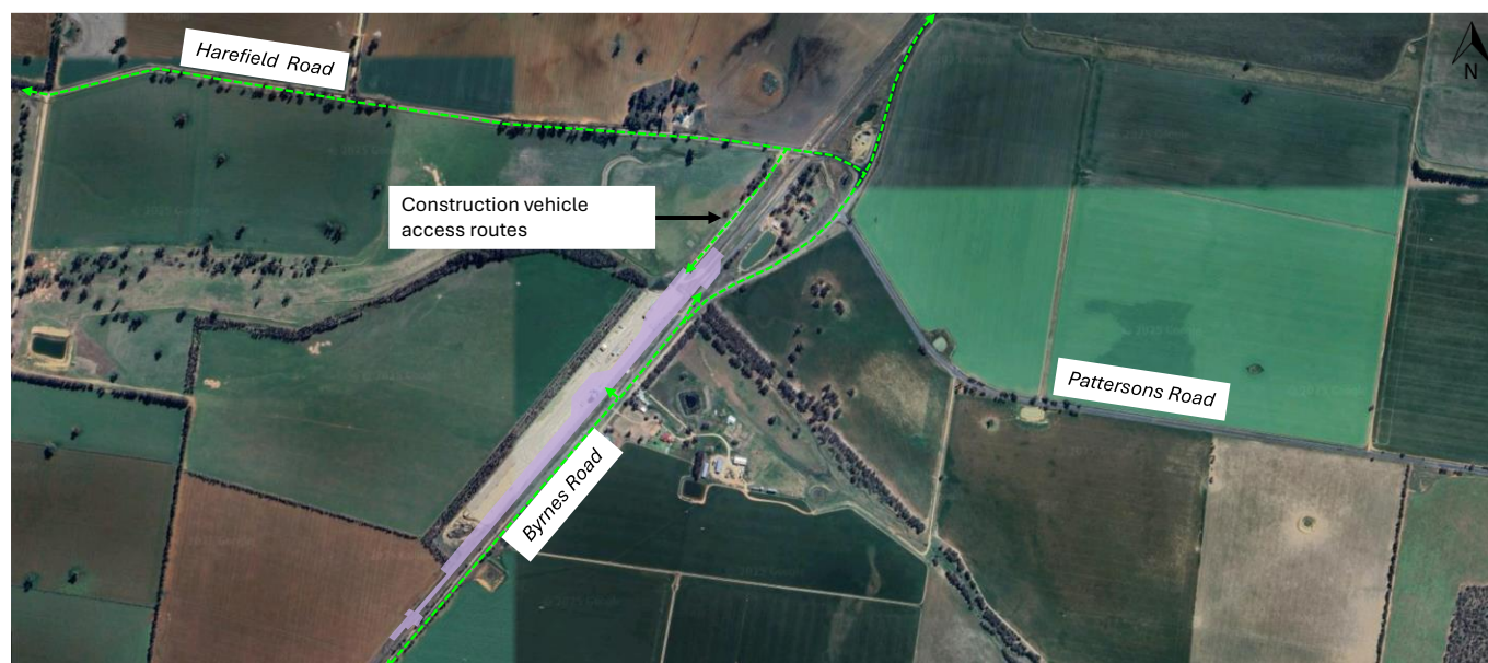
FIGURE 24: CONSTRUCTION VEHICLE ACCESS ROUTES – HAREFIELD YARD CLEARANCES
