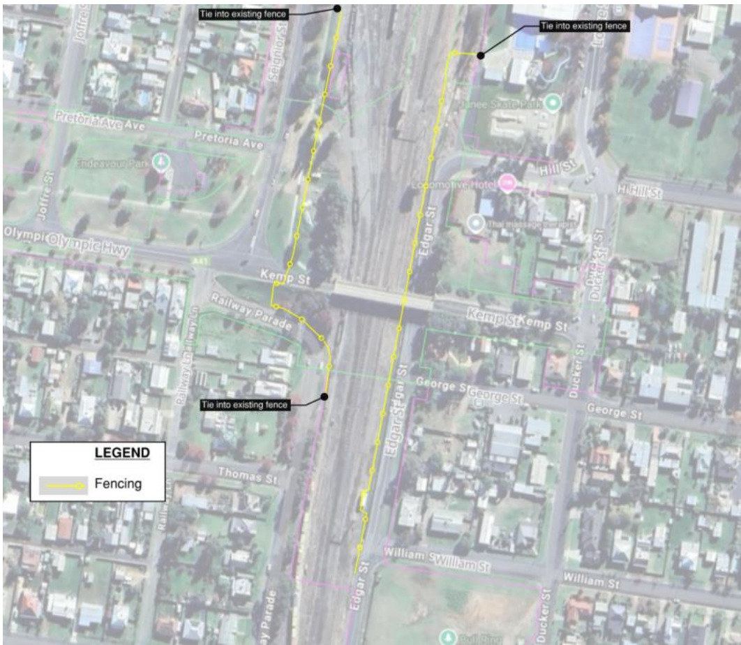
FIGURE 4 ALIGNMENT OF RAIL EXCLUSION FENCING INSTALLED PRIOR TO KEMP STREET BRIDGE CLOSURE
