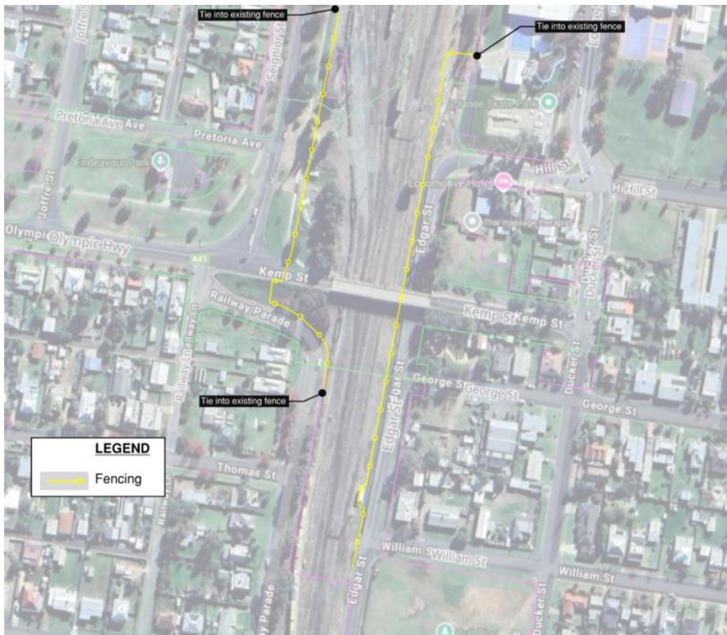
FIGURE 5 ALIGNMENT OF RAIL EXCLUSION FENCING INSTALLED PRIOR TO KEMP STREET BRIDGE CLOSURE
