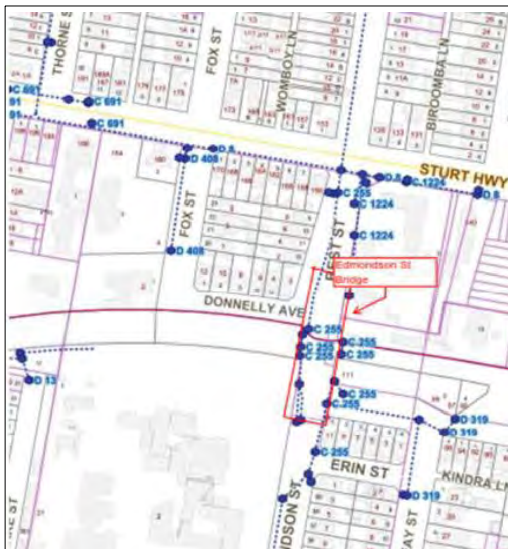
Figure 4.42 Estimated Wagga Wagga Council drainage based on historical records at Edmondson Street bridge
