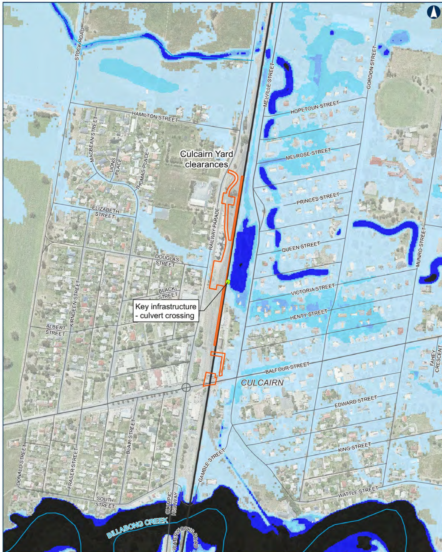
Figure 4.18 1% AEP flooding levels at the Culcairn Yard clearances enhancement site
