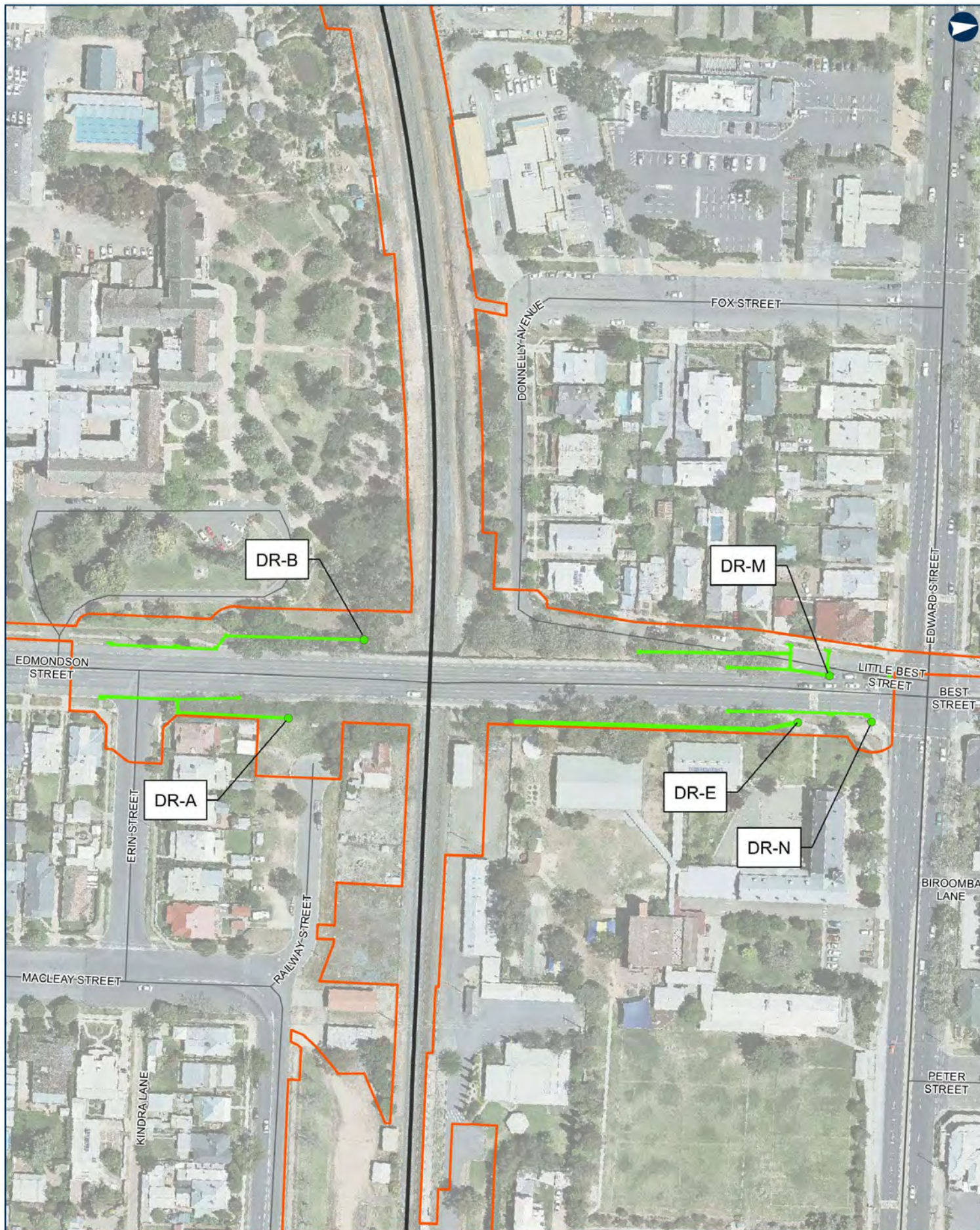
Figure 5.16 Edmondson Street bridge - proposed drainage
