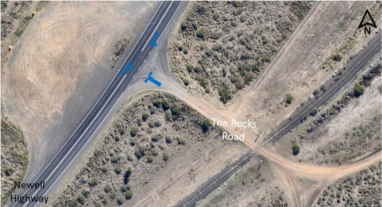
Figure 3-9 Newell Highway / The Rocks Road intersection layout and vehicle movements
