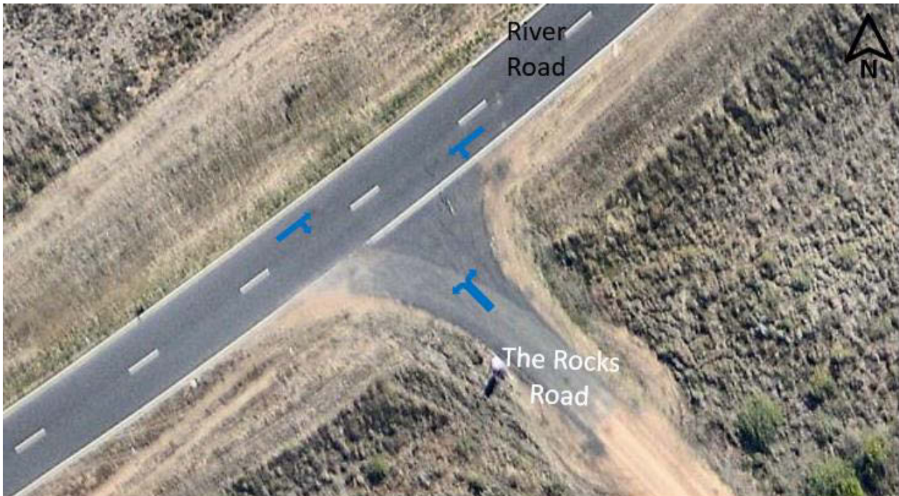
Figure 3-11 River Road(Back Pally Road) / The Rocks Road intersection layout and vehicle movements
