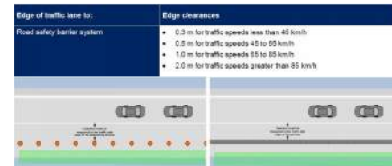
Figure 6-1: Clearance measurement from delineating device (system)
