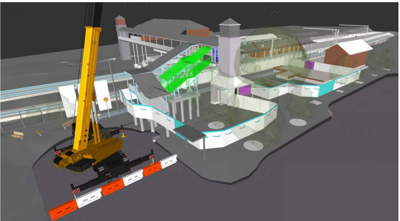
Figure 11 - Demolition of exiting stairs
