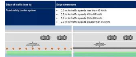
Figure 6-1: Clearance measurement from delineating device (system)
