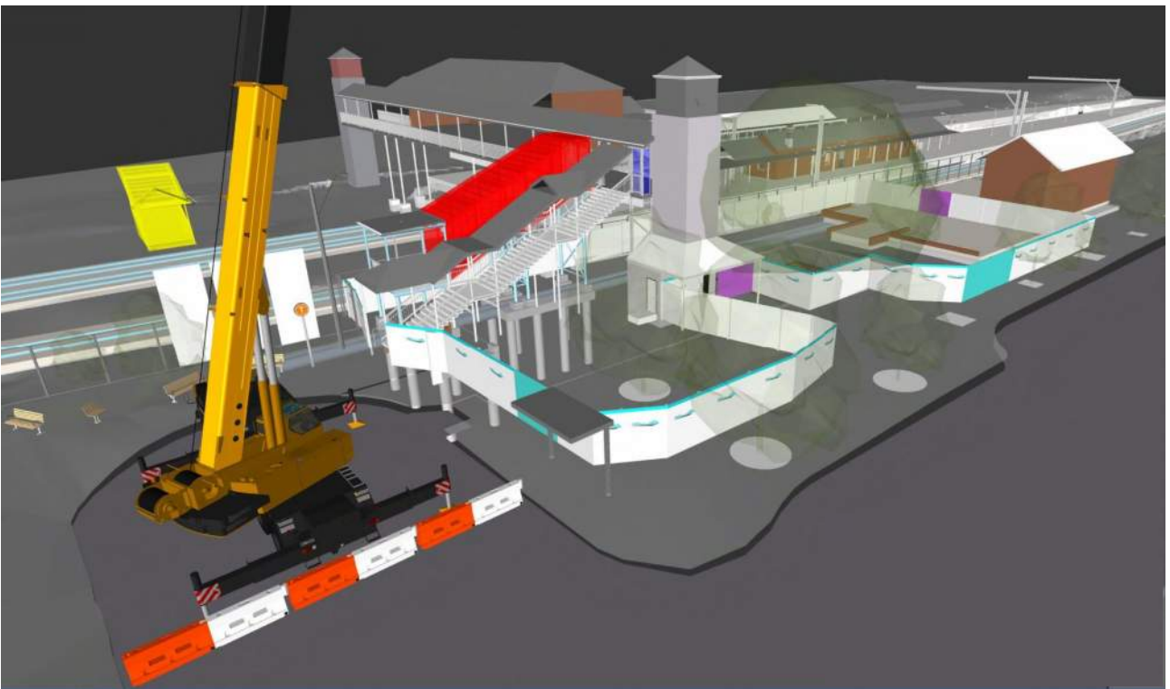
Figure 9 - Installation of new stair modules with 200t crane
