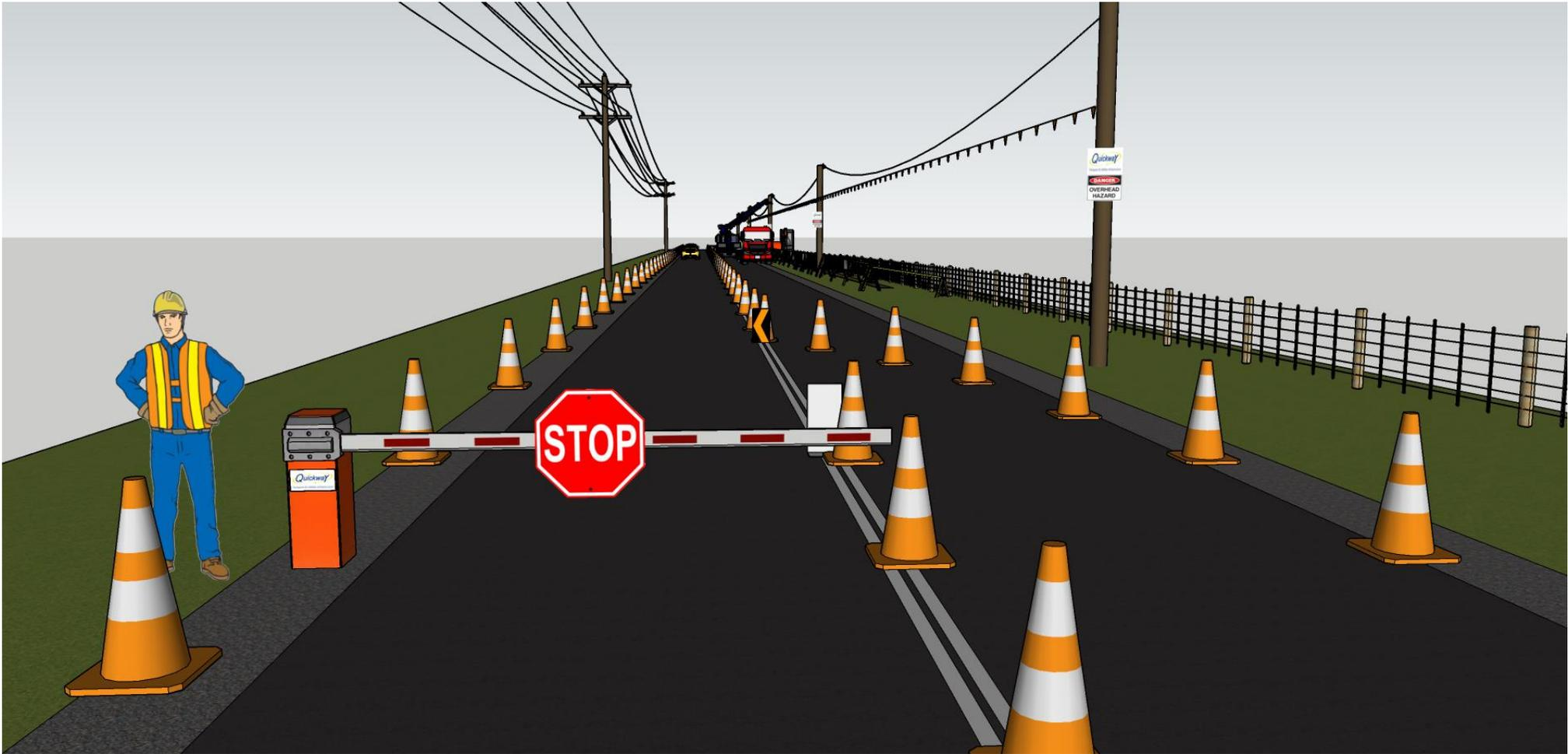
Figure 6.2 Example shuttle flow using portable boom barriers – short term site
