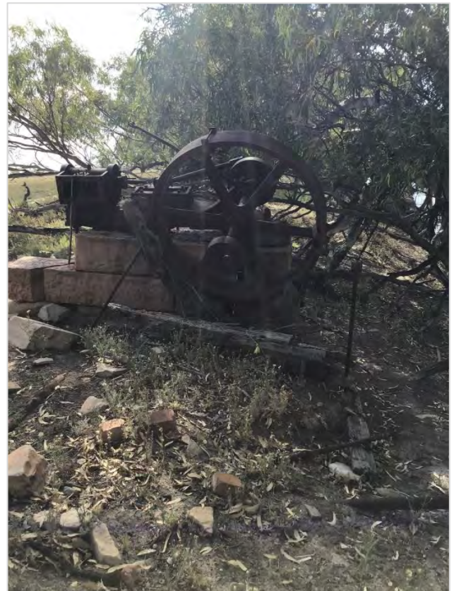
Figure 5-73 Reticulated piston and flywheel, remains of suction pipe in bottom right; facing east (Jacobs 2020)
